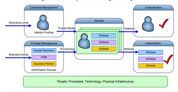
Figure 5. Basic Identity and Access Management Components
