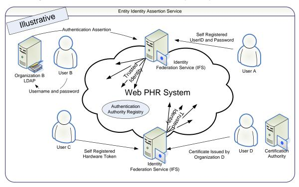
Figure 13. Illustrative Notional Architecture for Entity Identity Assertion Service
