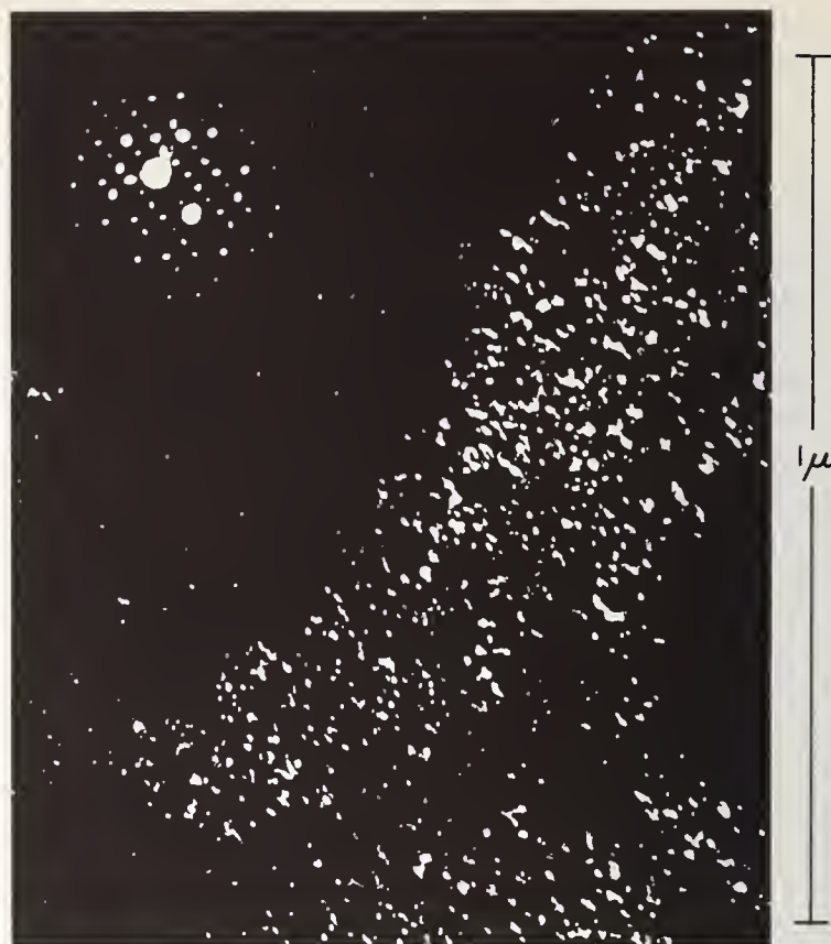
FIGURE 7. Dark field electron micrograph showing \omega -phase in Ti-Mo (5 at.%).
