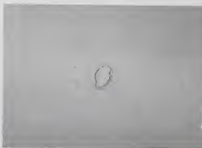
Figure 5 Detail of ZnSe film grown on GaAs at 192^\circ\text{C} . Magnification is as figure (3).
