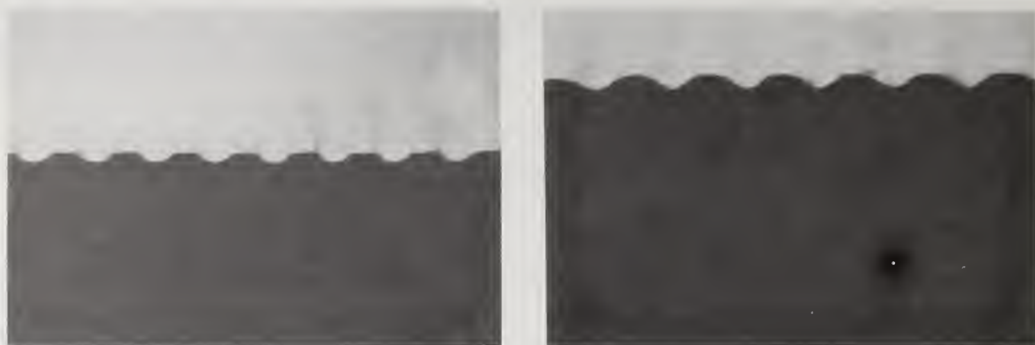
Figure 4. Photomicrographs of two holographic gratings illustrating groove profiles. Groove spacing on the left is 1800 \ell/\text{mm} and on the right is 1200 \ell/\text{mm} .
