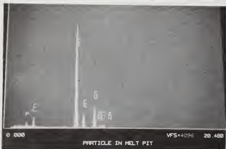
Figure 7. EDX spectra of one of the particles in figure 6 showing a high concentration of iron and trace amounts of phosphorus and zinc.
