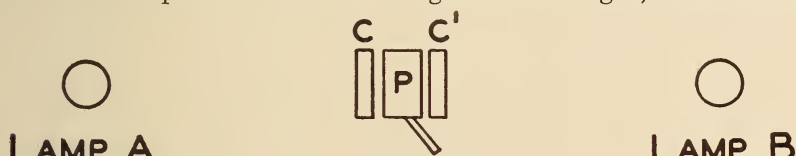
FIGURE 33.—Schematic diagram showing photometer used to test the color match of the lamp-and-filter combinations
