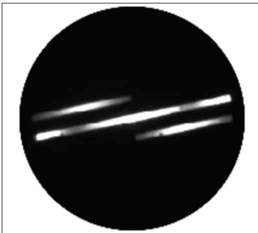
Figure 3. Image of the back focal plane of a microscope with a tilted slit illumination, showing angle-resolved specular (zero order, longer line) and diffracted (first order, shorter side lines) efficiencies.
