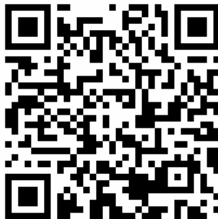
Figure 2 - A QR code example which has encoded the text “NISTIR 8202 - Blockchain Technology Overview QR code example”
