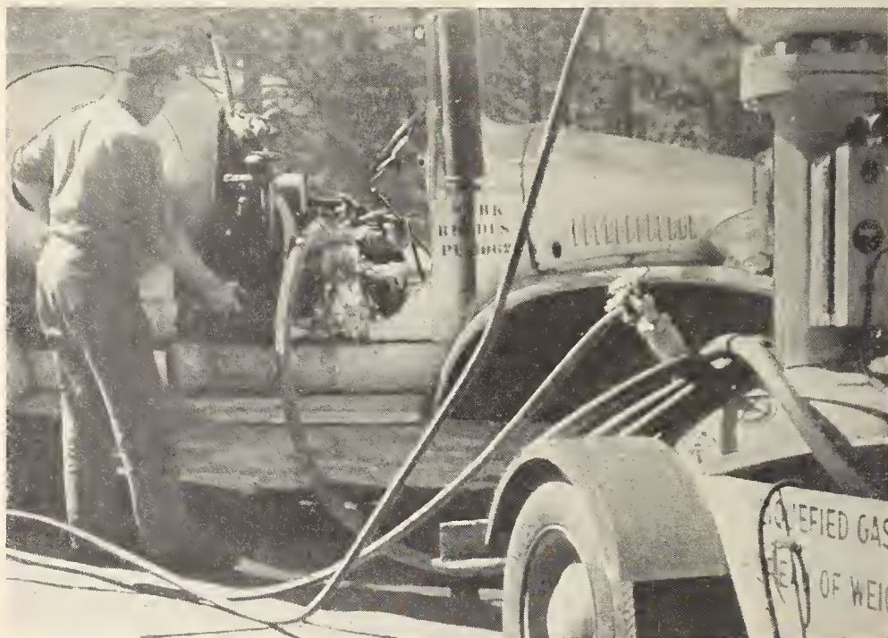
FIGURE 10. Testing a truck meter with State of California prover.
