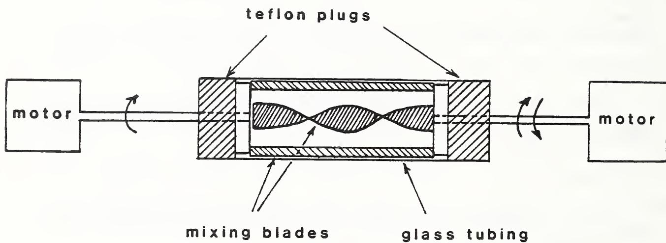
Figure 1. A diagram of the mixer is shown. The twisted blade, which rotates on the central axis of the mixer, is driven by the bi-directional motor. Three blades, driven by the uni-directional motor, are at the outer circumference of the mixer, near the glass wall; one of these is a scraper which prevents accumulation of material at the wall.
