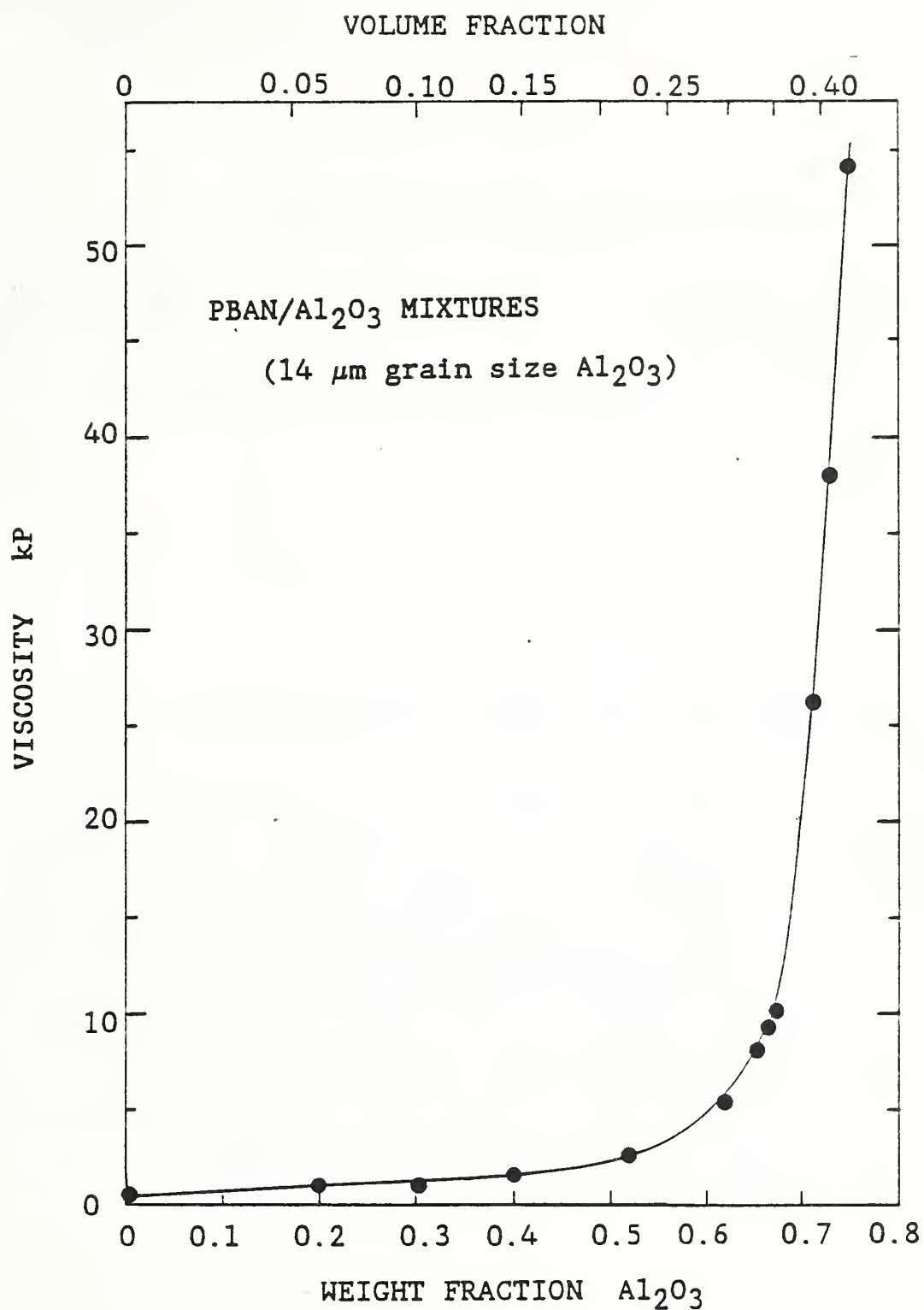
**Figure 10.** Viscosity vs concentration for aluminum oxide filled PBAN is shown. The measurements are reported for a shear rate of 0.55  $s^{-1}$ .
