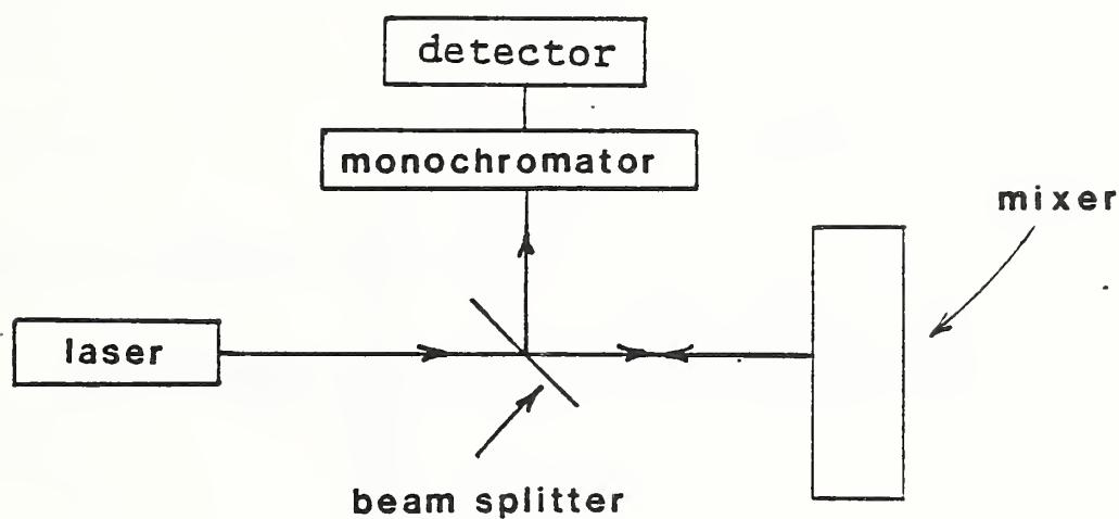
Figure 2. The optical arrangement for the fluorescence mixing experiment is shown. By using a beam splitter, the back scattered fluorescence is measured.
