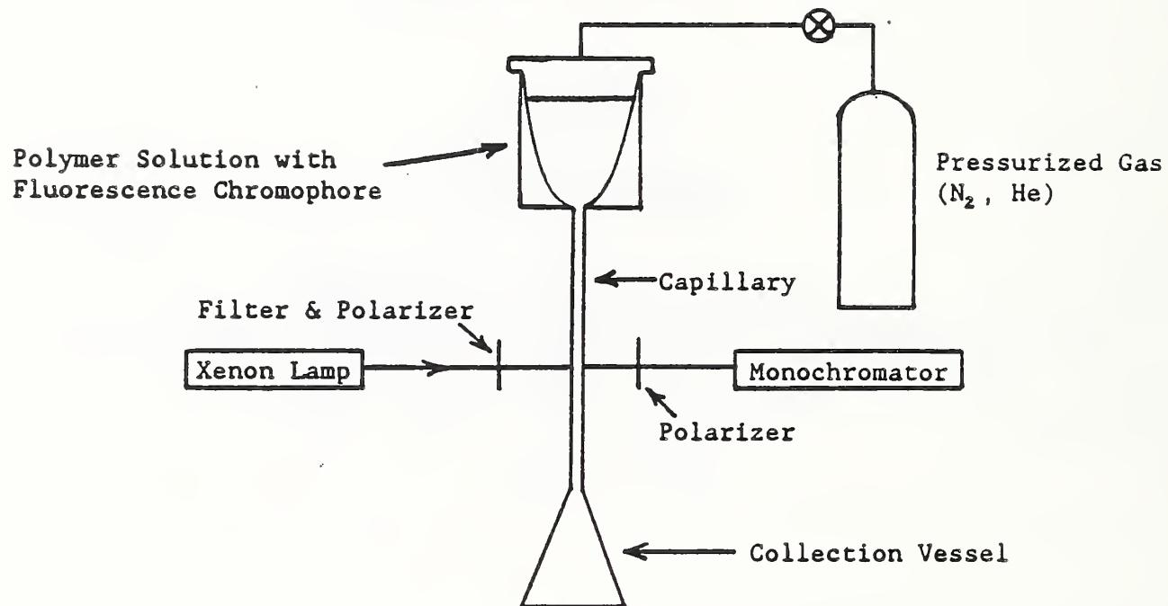
Measurement: Fluorescence Anisotropy as a Function of Shear Rate or Applied Pressure.
