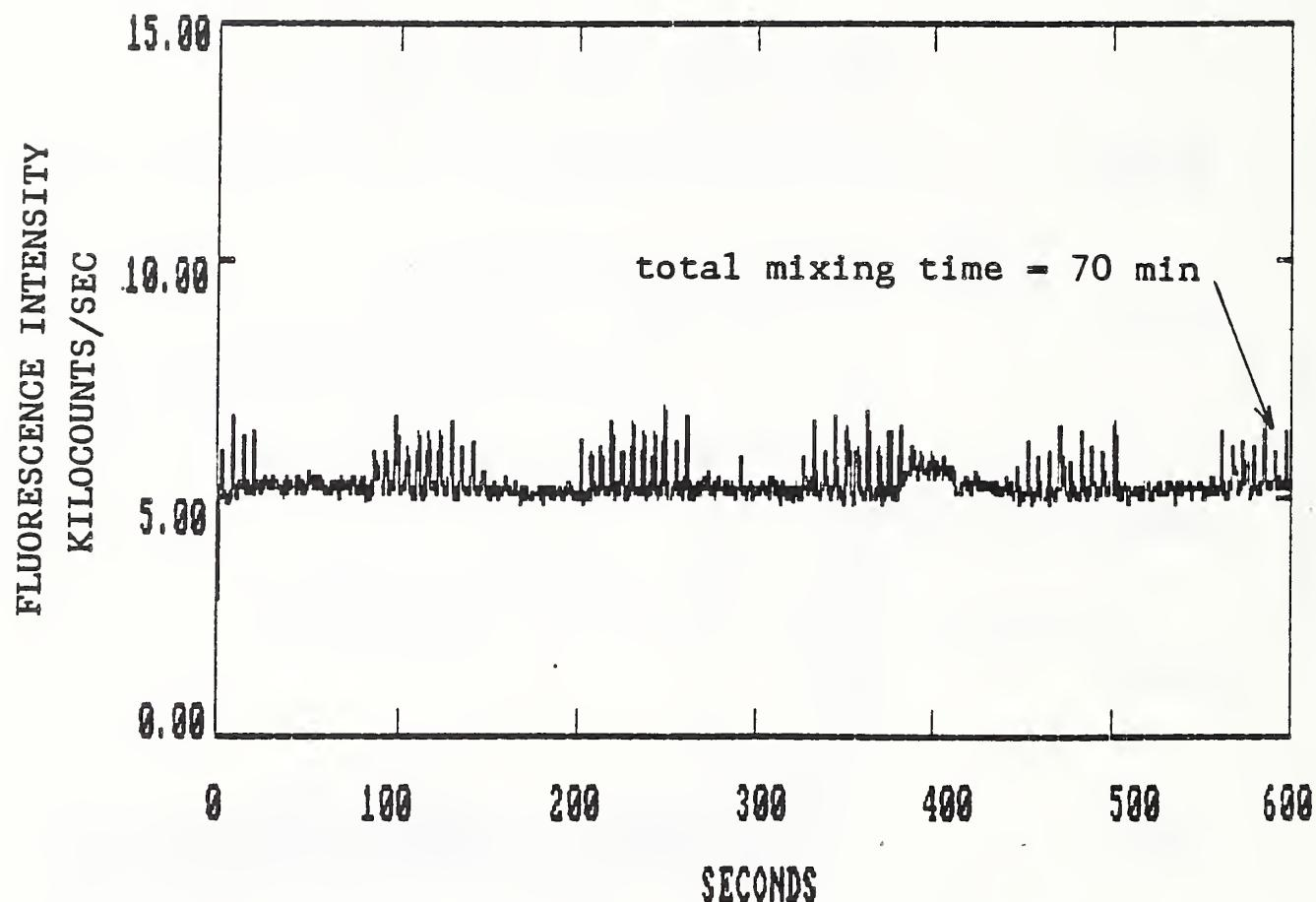
Figure 5. Fluorescence intensity versus time is plotted for mixing of coumarin 30 doped PBAN with 58% aluminum oxide by weight. This is the same specimen as was used for the data in Figure 4. The observations are for mixing times starting at 60 and ending at 70 minutes.
