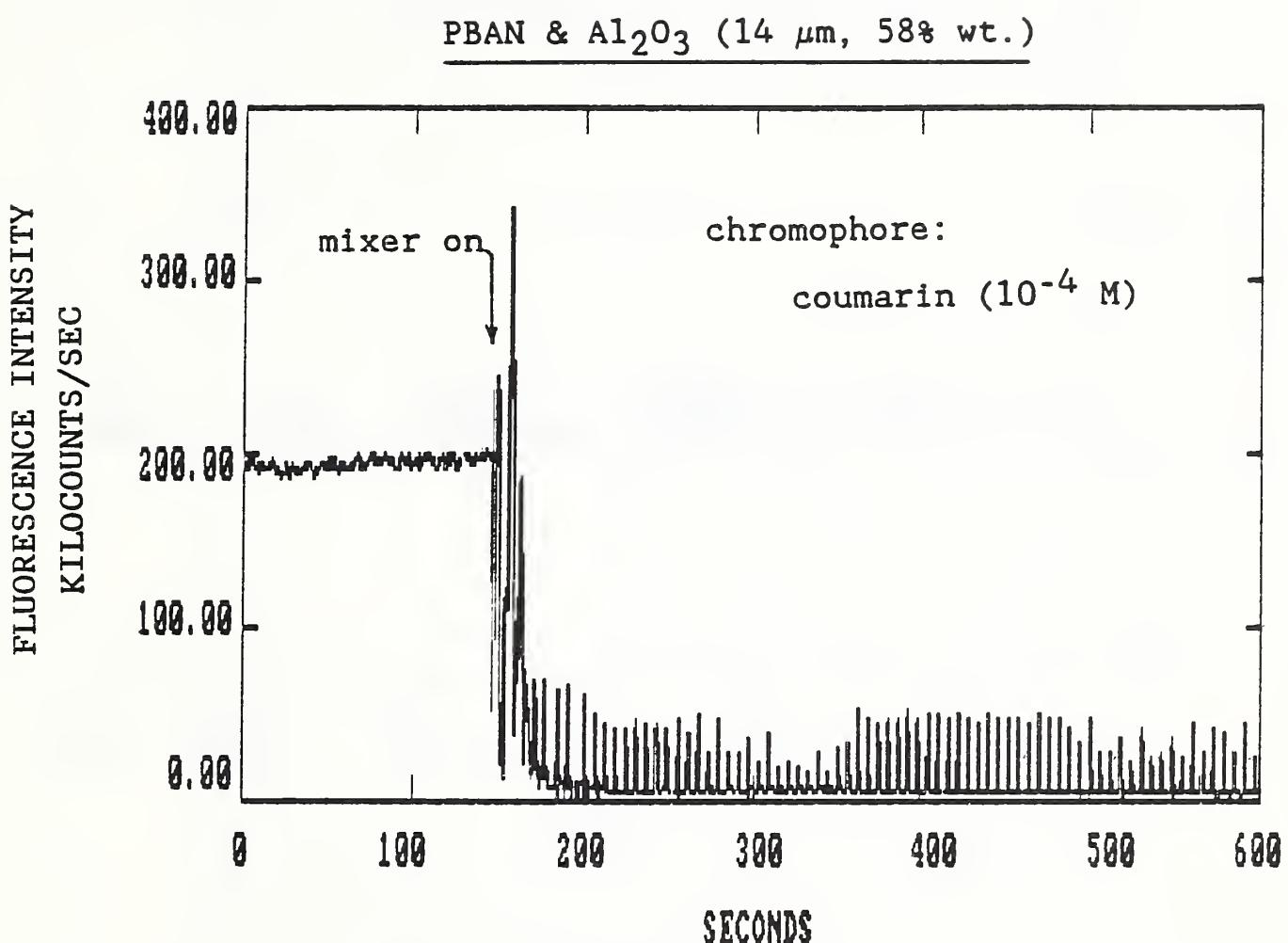
**Figure 4.** Fluorescence intensity versus time is plotted for mixing of coumarin 30 doped PBAN with 58% aluminum oxide by weight. Grain size of the aluminum oxide was 14  $\mu\text{m}$ .
