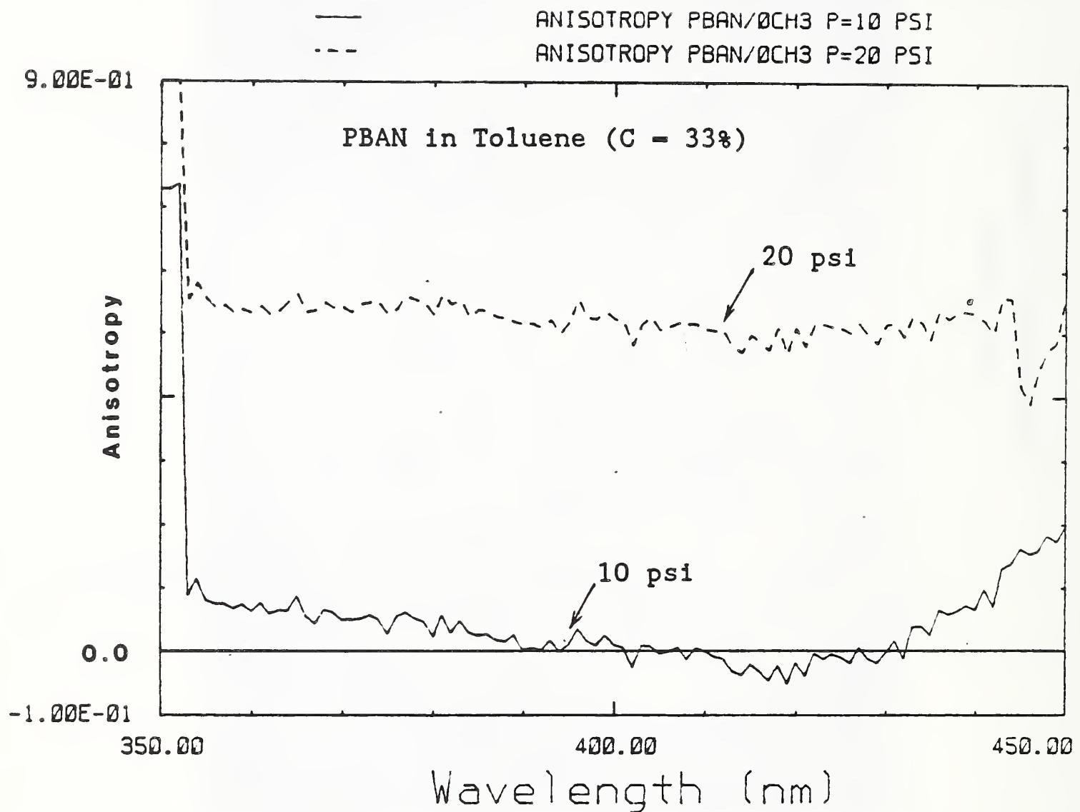
Figure 9. The fluorescence anisotropy for a concentrated solution of PBAN in toluene is shown for a wavelength scan of 350 to 450 nm for 10 and 20 psi capillary head pressures.
