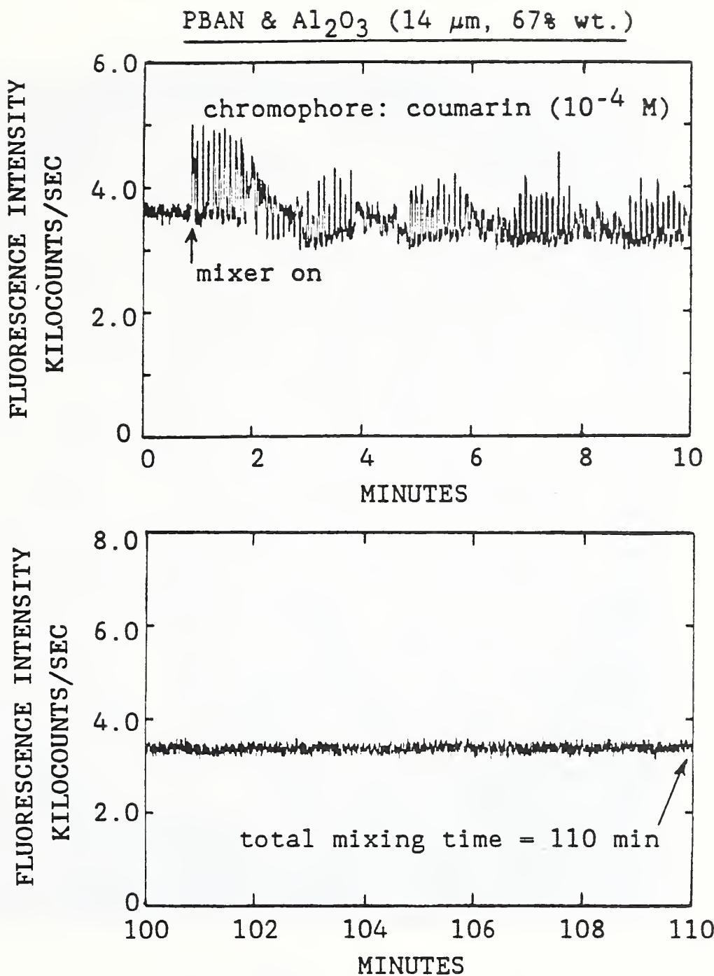
Figure 6. Fluorescence intensity versus time is plotted for mixing of PBAN with 67% aluminum oxide by weight. The starting specimen was that used for the data of Figures 4 and 5 to which more aluminum oxide was added. The plot for 0 to 10 minutes shows the intensity variations at the beginning of mixing. The plot from 100 to 110 minutes shows the intensity at the end of mixing.
