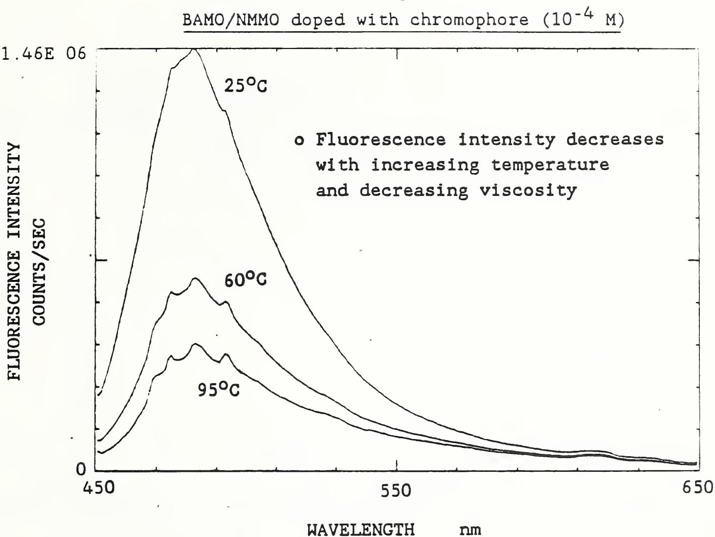
Figure 8. The fluorescence spectra of a doped polymer binder, BAMO/NMMO, are shown for 25, 60, and 95°C. The chromophore was p-dimethylaminobenzylidene malononitrile.
