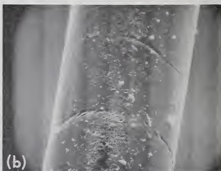
FIGURE 7. Electron microphotograph of platinum thermometer wire subjected to a total of several hundred hours at 420 °C. Magnification: photograph (a) 172× (b) 850×. The photographs show: (1) grain growth; (2) migration. No attempt has been made to date to identify the white "hecks."
