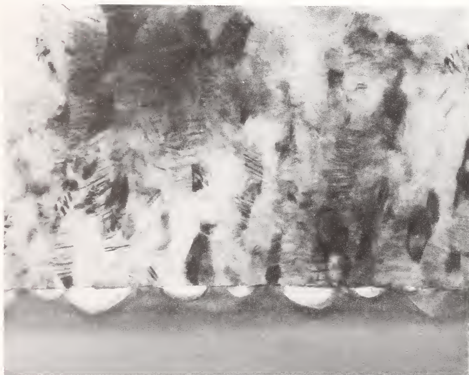
Figure 7 Cross sectional TEM image taken of ZnS film at periphery of laser damage site. Degree of melt back of ZnS induced by heating effect of laser driven plasma is clearly shown
