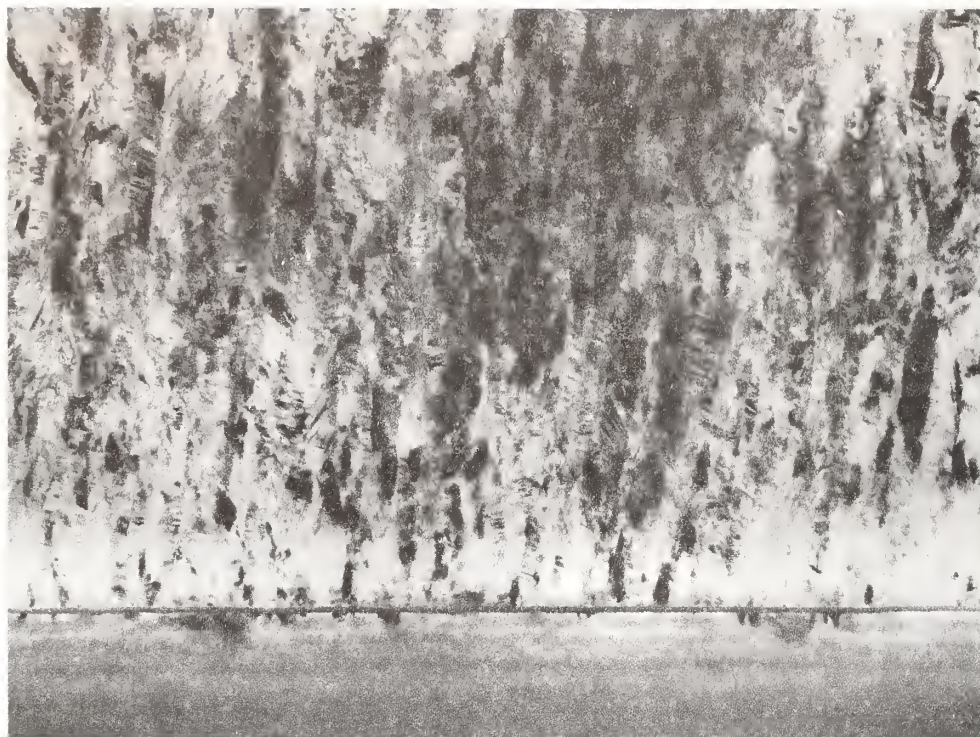
Figure 1 Polycrystalline ZnS film deposited in UHV on germanium
