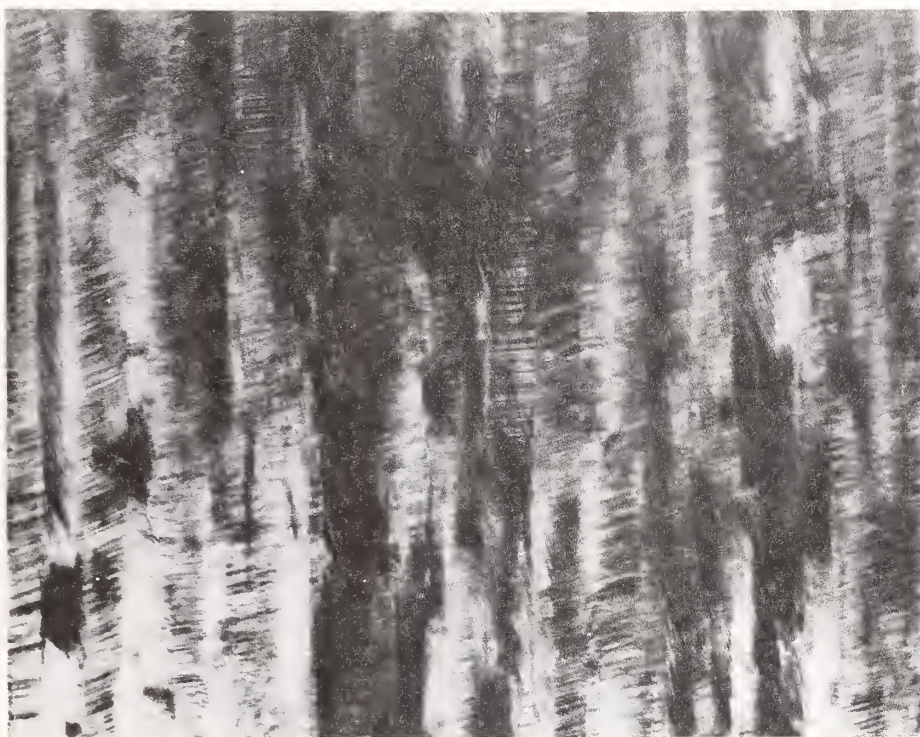
Figure 3 Microstructure of alloyed \text{ZnS}_x\text{Se}_{1-x} film on glass substrate
