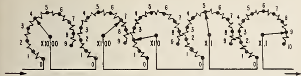
FIGURE 36. Schematic diagram of rheostat arm of bridge.
