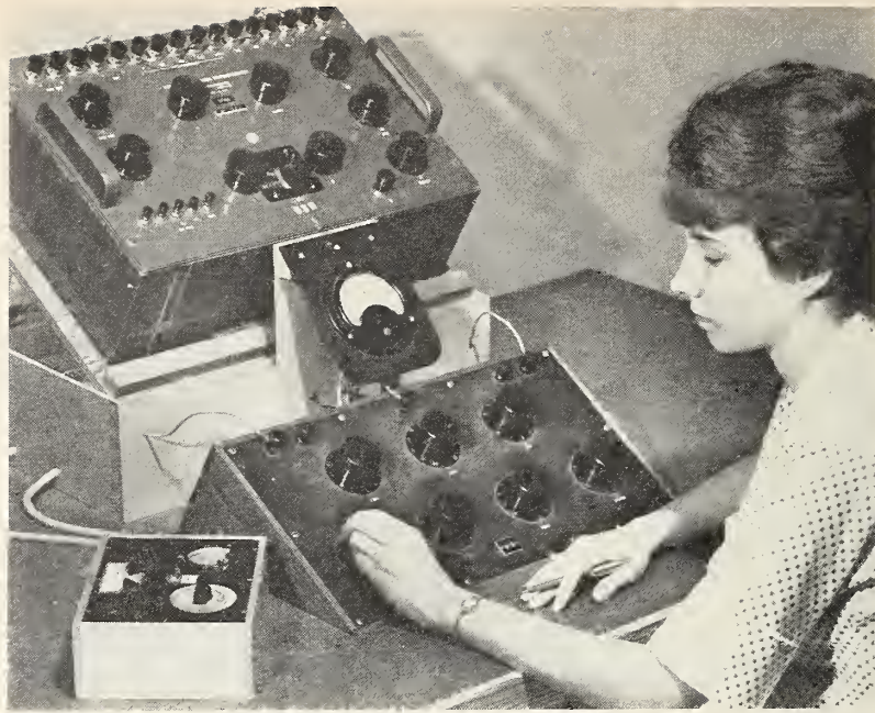
Universal Ratio Set connected for calibration of a potentiometer.
