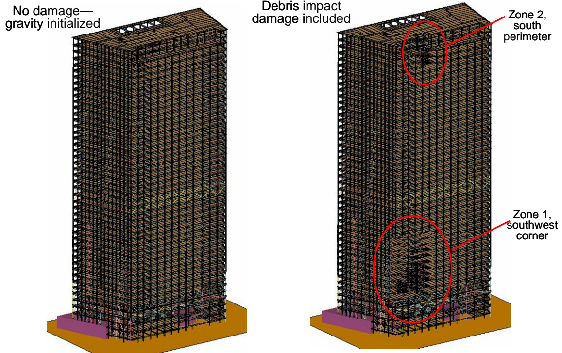
Figure 3-52. WTC 1 debris impact damage application to the global LS-DYNA model.
