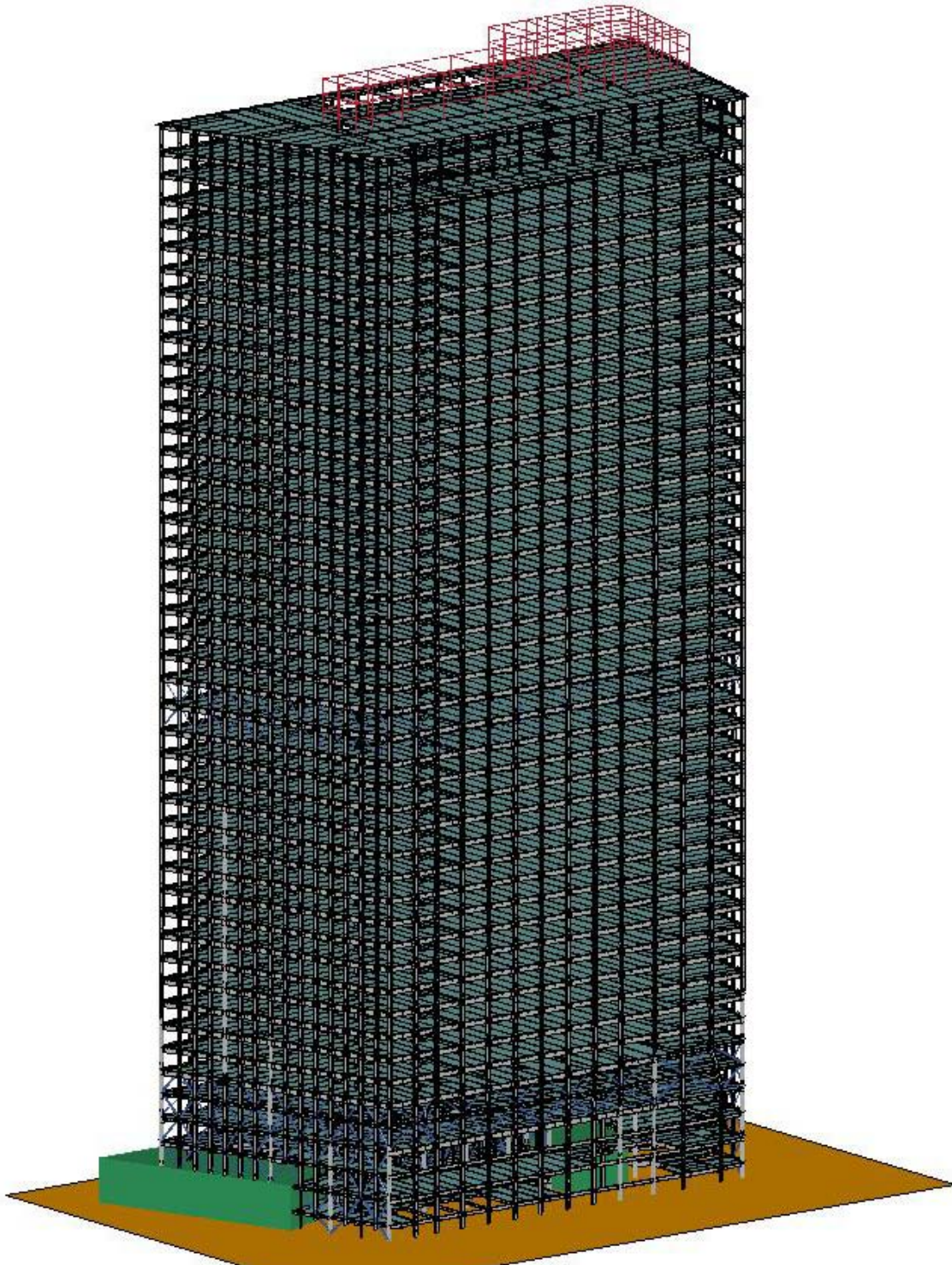
Figure 3-20 Global model of WTC 7, viewed from the southwest.
