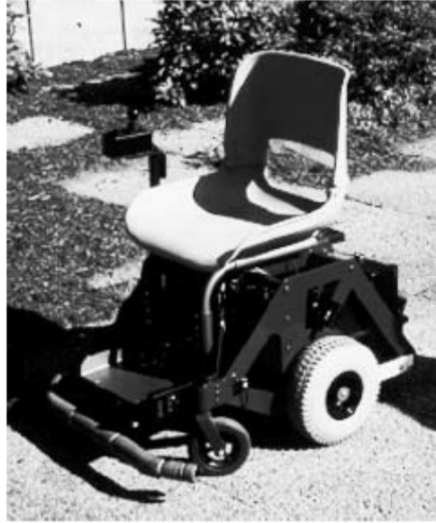
Figure 3 Wheelesley , the robotic wheelchair system.
