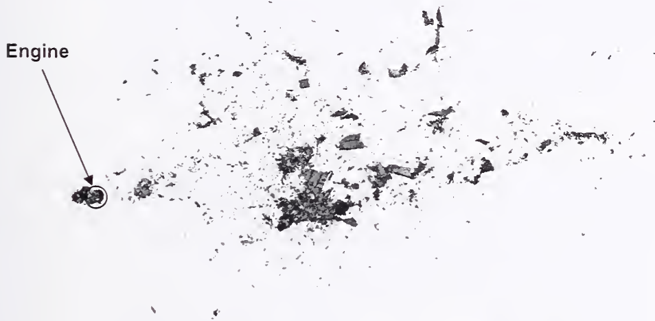
(b) Aircraft debris field (time=0.715 s)
