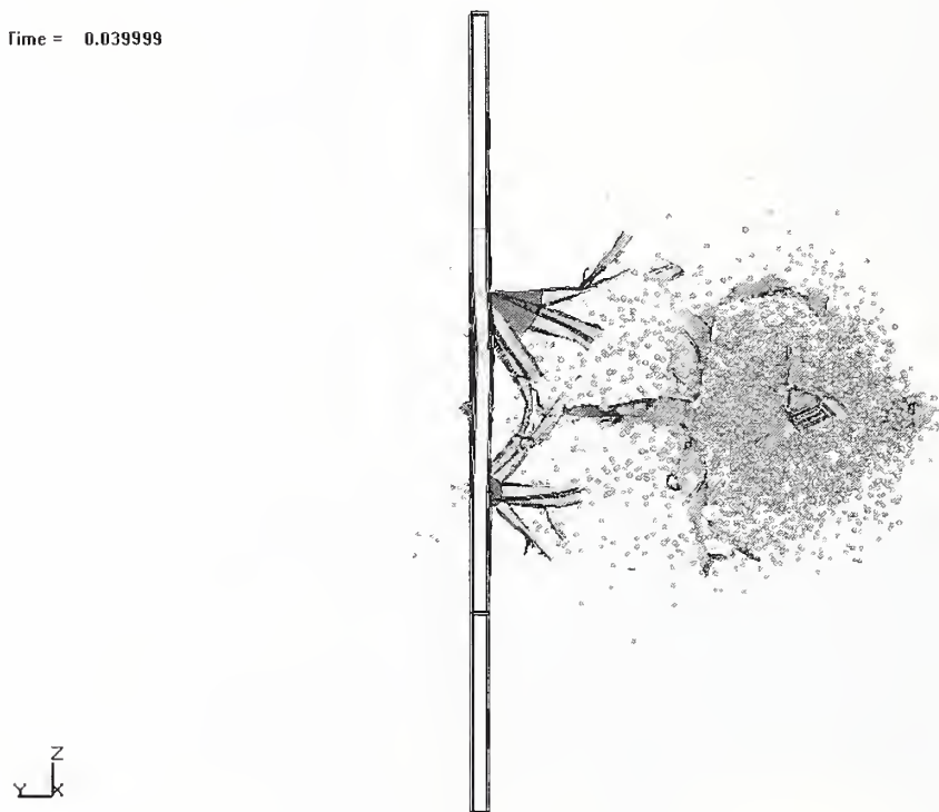
Figure 5-47. SPH analysis of structural damage and fuel dispersion (side view).
