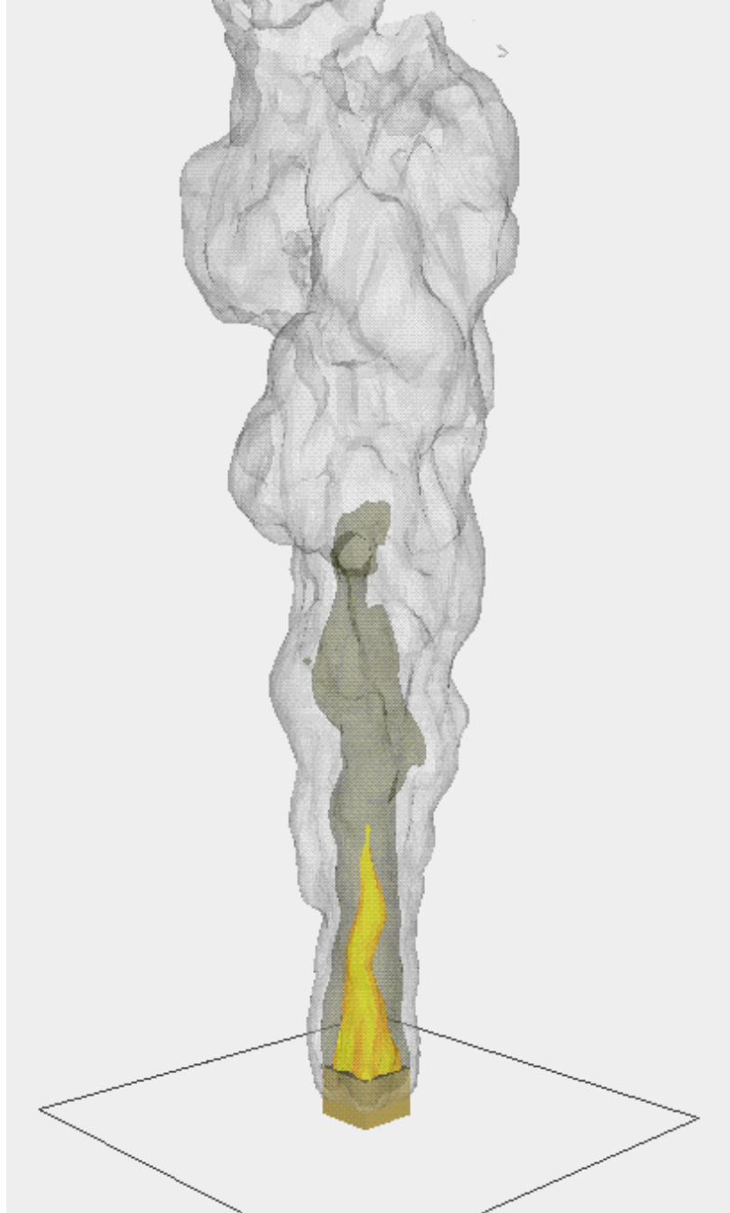
Figure 1: Instantaneous snapshot of a pool fire simulation. The contours correspond roughly to the boundaries of the continuous flame, intermittent region and plume. The square burner is 0.2 m by 0.2 m, the dimensions of the computational domain are 1.5 m by 1.5 m by 3.5 m.
