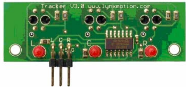
Fig. 6. Lynxmotion Line Tracker
