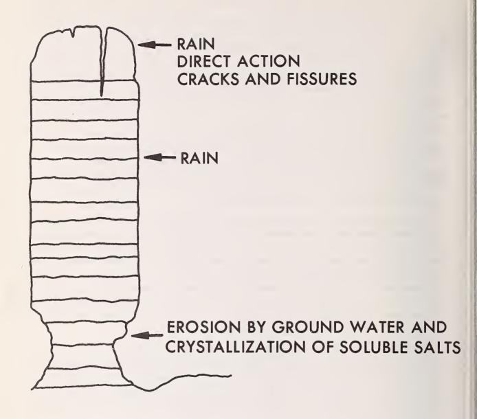
Figure 2. Deleterious Action of Water on Adobe Walls.
