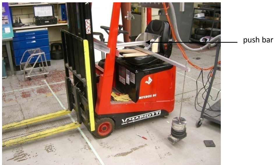
Figure 5. Applying (a) horizontal and (b) vertical forces. The spring scale shown in (a) indicates the applied force on the SIP device.
