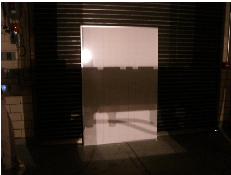
Figure 11. Shadows on the test screen when fork arms were raised to 117 cm
