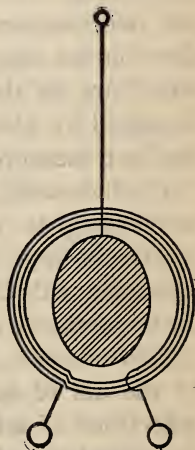
FIG. 117.—Type of electrodynamometer suitable for radio current measurement
