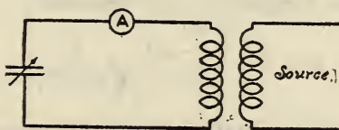
FIG. 128.—Circuit for measuring resistance by the reactance variation method
