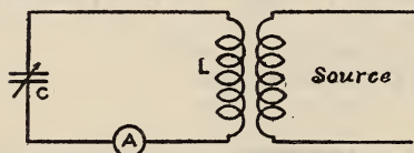
FIG. 134.—Coil resistance measurement in terms of known circuit or standard coil
