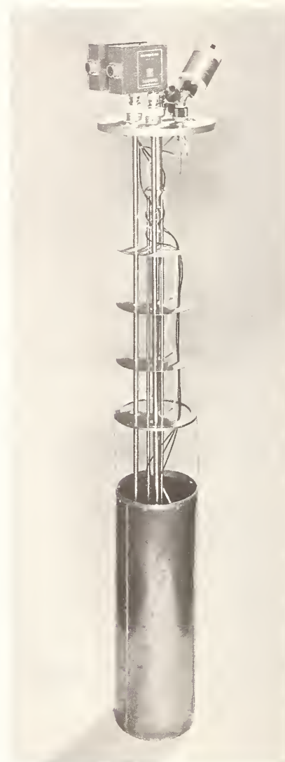
FIGURE 5(a). Overall view of cryogenic apparatus. The Dural block at the top is an electromagnetic and thermal shield for the potential leads, and the niobium can surrounding the comparator and flux transformer is a superconducting shield.
