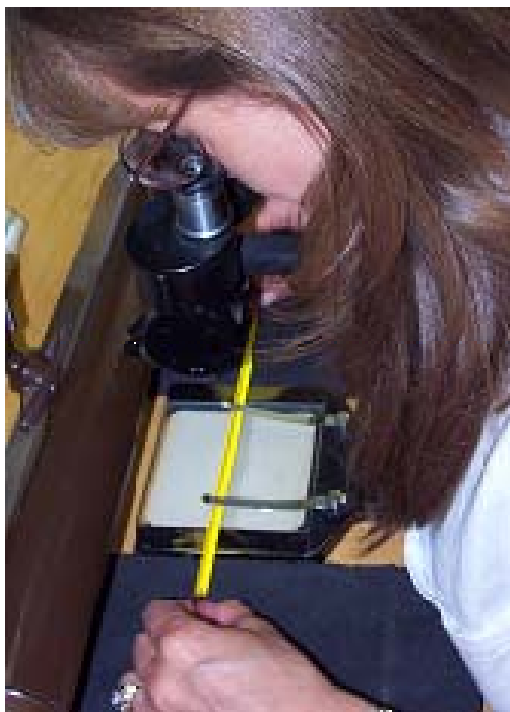
Fig. 4. Visual inspection of a liquid in glass thermometer using a low-power microscope (10X).
