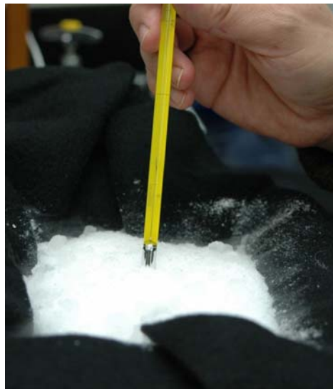
Fig. 5. The bottom portion of a mercury thermometer bulb is being cooled in dry ice to join a separated mercury column. Note: to prevent breakage, do not let the mercury freeze in the thermometer bulb.
