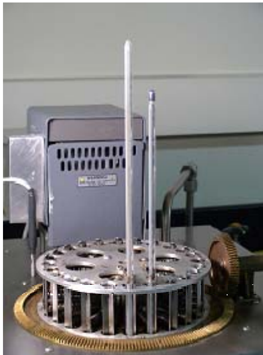
Fig. 6. Heating a mercury thermometer upside down in a liquid bath near 250 °C to join a separated mercury column. A second thermometer is used to monitor the bath temperature.
