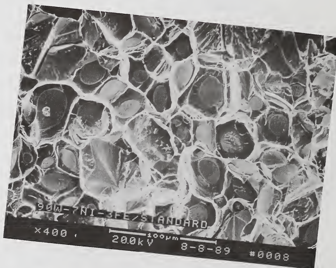
Figure 2. SEM micrograph of the fracture surface of the as-sintered 90W-7Ni-3Fe heavy alloy.
