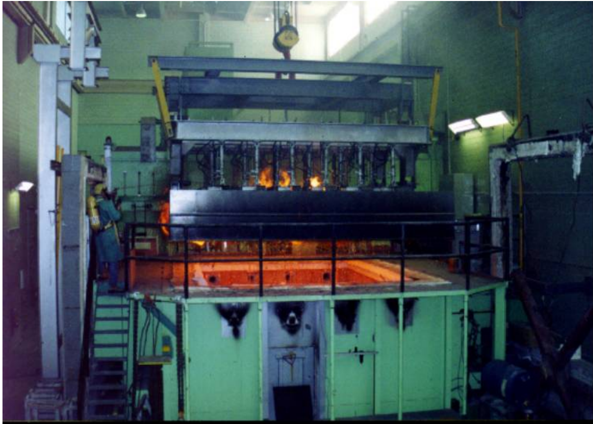
Figure 6. Photograph of modern floor testing furnace (Kodur)
