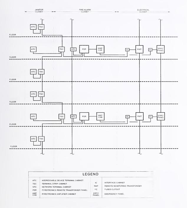
Figure 5-20. Fire alarm closet with PSR location.
