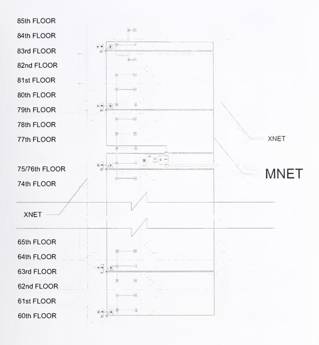
Figure 5–22. Locations of typical MNET network equipment.
