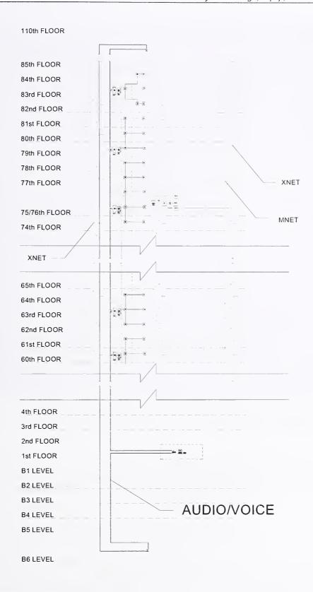
Figure 5-28. Locations of audible notification appliance network equipment.
