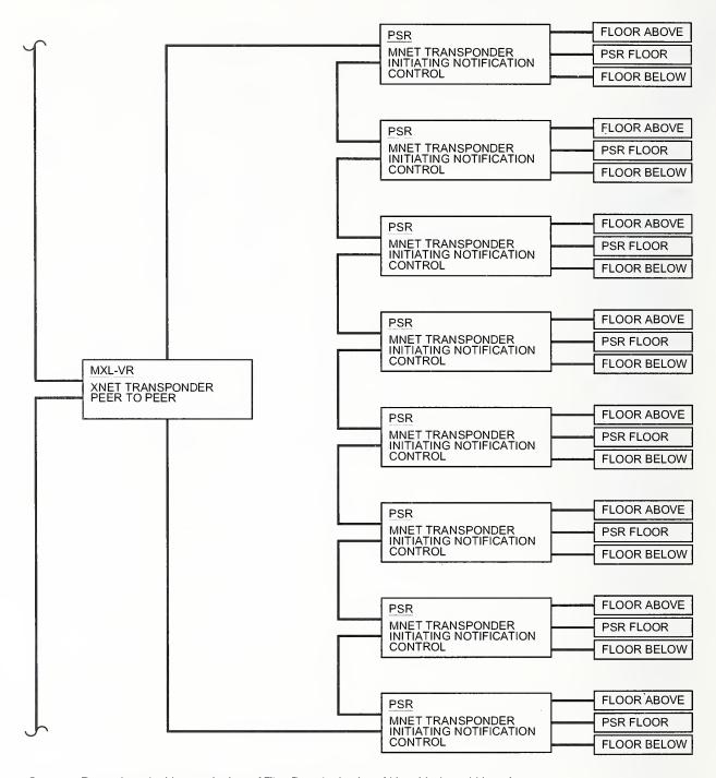
Figure 5–21. Single-line schematic of MNET network configuration.
