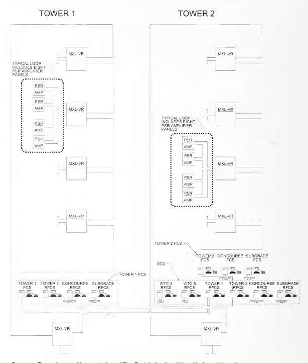
Figure 5–27. Single-line schematic of notification appliance network.
