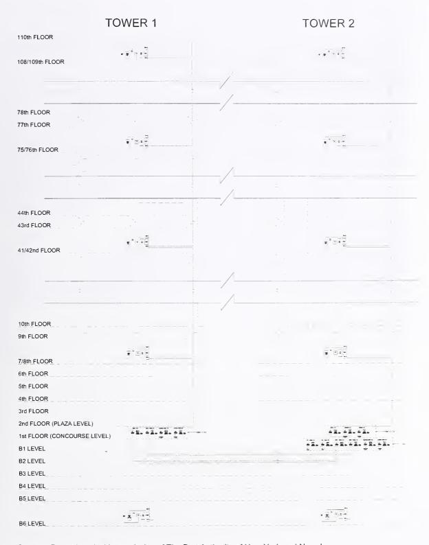
Figure 5–24. Locations of XNET network equipment.
