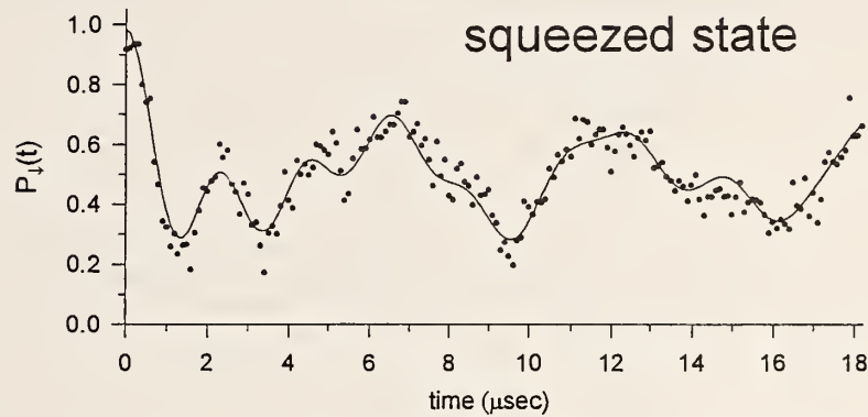
Figure 6. P_1(t) for a squeezed state. The data are fitted to a squeezed state population distribution, yielding \beta \approx 40 \pm 10 (16 dB below the zero point variance), which corresponds to \bar{n} \approx 7.1 .
