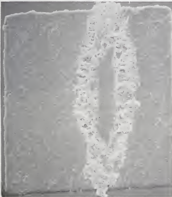
Fig. 3-14. SEM photomicrograph of the lift-off pattern of a normal bond made under laboratory conditions. The pattern, which clearly reveals the unwelded center portion of the bonded region, was exposed by carefully peeling back the bond. Magnification: 510 x.
