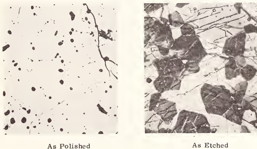
FIGURE 2 Microstructure of U_{0.495}C_{0.485}O_{0.02} (UCON-283) Before and After Thermal Diffusivity Measurements to 1500°C. The Oxycarbide is Single Phase with a Trace of Free Uranium (White Phase). 281X
