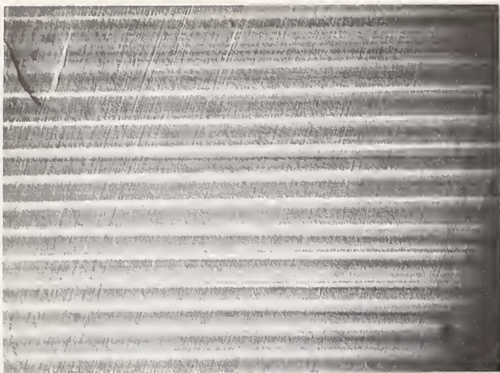
Fig. 5. Top view of the surface of the epitaxial layer shown in Fig. 4. The surface was etched in B-etch to reveal the arrays.
