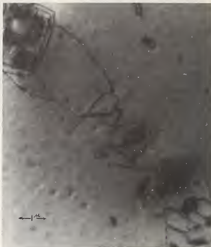
Fig. G.2. Observe dislocation generation around \text{SiO}_x complexes. Dislocations were found purely edge-type. TEM observation, courtesy of Patrick and Dash.
