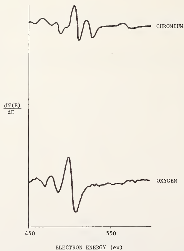
Figure 8 Auger Spectra of Chromium and Oxygen
