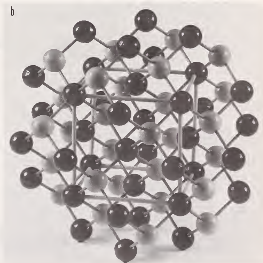
Fig. 6. Views of a diamond-type lattice from (a) a \langle 110 \rangle direction, and (b) 10^\circ off a \langle 110 \rangle direction.
