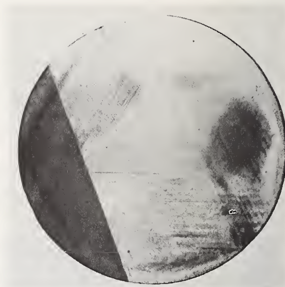
Fig. D.2b. Epitaxial film over polished region is highly defective as evidenced by strong diffraction contrast.
