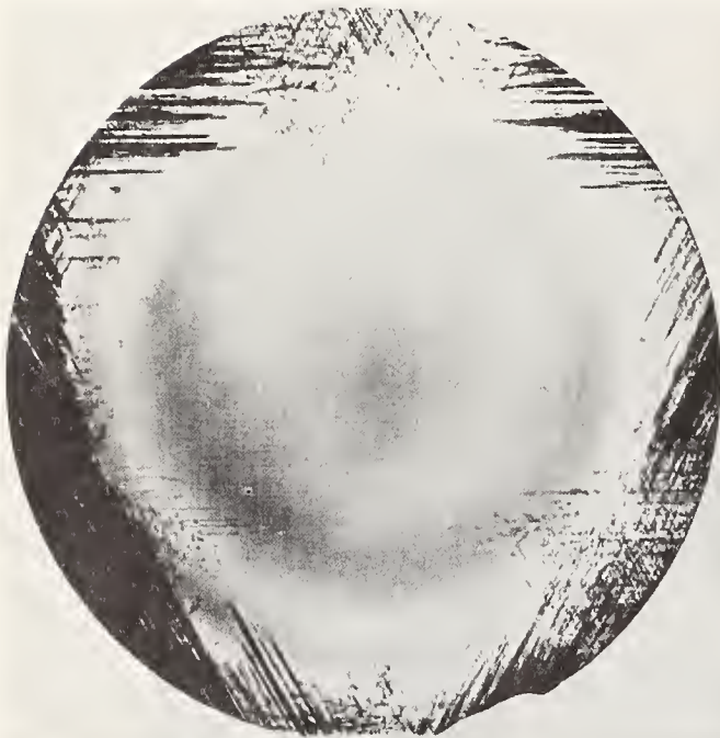
Fig. 6. Topograph of silicon wafer showing process-induced defects.
