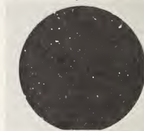
Fig. 3 - SiO 2 Deposit on inadequately cleaned silicon. Oblique illumination.
