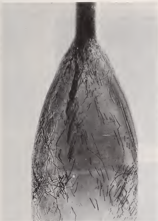
Fig. 10. Topograph of crystal section showing dislocations propagating from seed into body of crystal.
