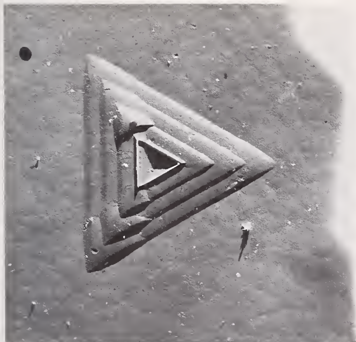
Fig. D.4. Replication electron micrograph of a stacking fault.
