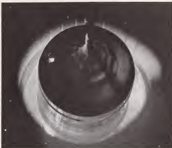
Fig. 2. Large diameter (4-1/2") silicon crystal being grown.
