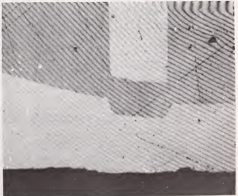
Fig. 10. Emitter-dip effect in n-p-n structure, photograph courtesy of R. J. Jaccodine.
