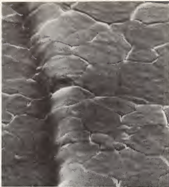
Fig. 4. Good Metal Step Coverage.
