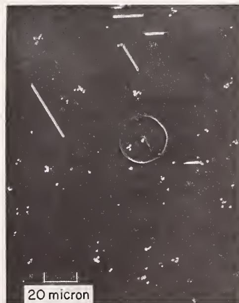
Fig. 7. Etch figures produced by a 2-minute Dash etch on a sample in which the oxygen was precipitated by annealing at 1100\text{ }^{\circ}\text{C} for 50 hours. Resistivity was 11.8\Omega\text{cm} ; boron doped; initial oxygen concentration of 12.9 \times 10^{17} atoms/cc.
