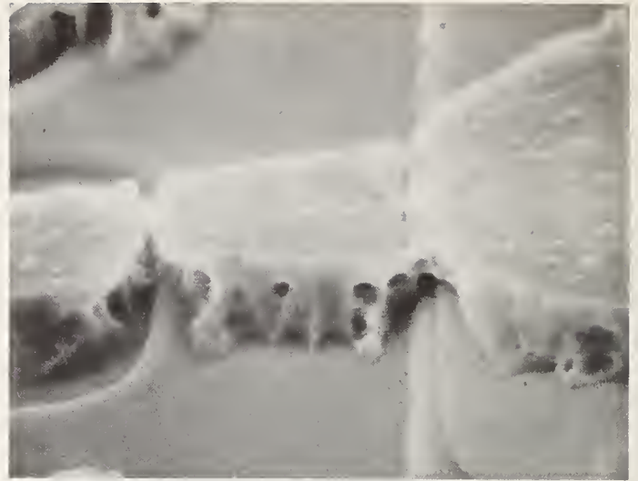
Fig. 5. Damage Due to Etchant Entering Step Defect.
