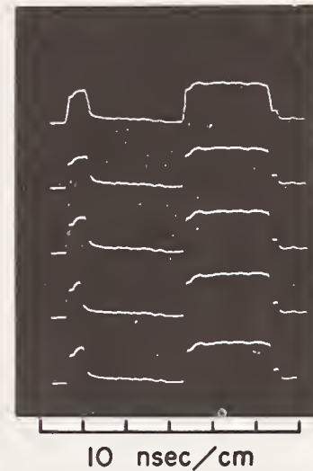
Figure 10. Typical damage data for an absorbing sample. The time until termination of the pulse transmitted through the sample (that pulse on the left of each trace) is proportional to the pulse intensity. The upper trace has been re-touched on the rise and fall of the pulses.
