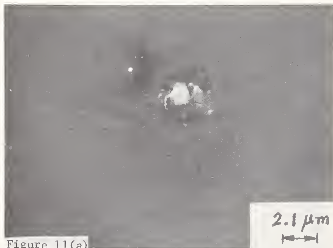
Figure 11. (a) SEM photograph of a large damage site on \text{YVO}_4 surface; a spark was observed and the spot-size is 160 \mu\text{m} . (b) Close-up view shows that the damage is due to a nonmetallic inclusion, 1.2 \mu\text{m} in diameter, which was about 0.2 \mu\text{m} below the plane surface. The morphology has crack nucleation similar to that in reference 8.
