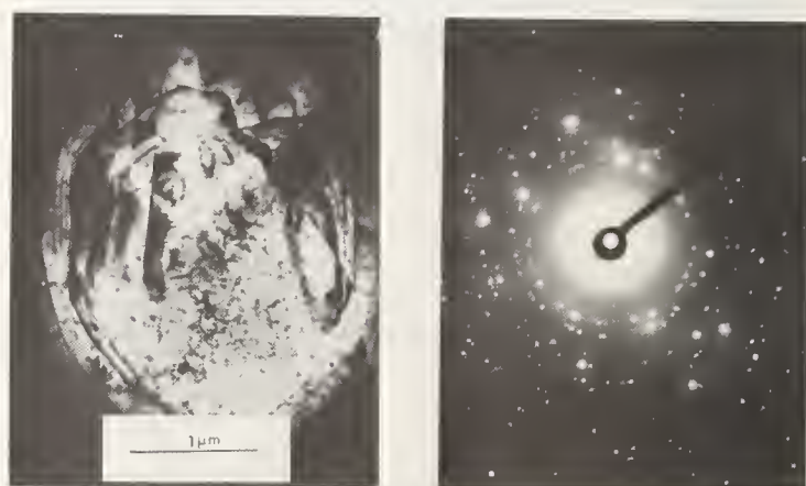
Figure 11. Structure of a sputtered Ge film surrounding the 10.6 \mu\text{m} laser damaged region.
