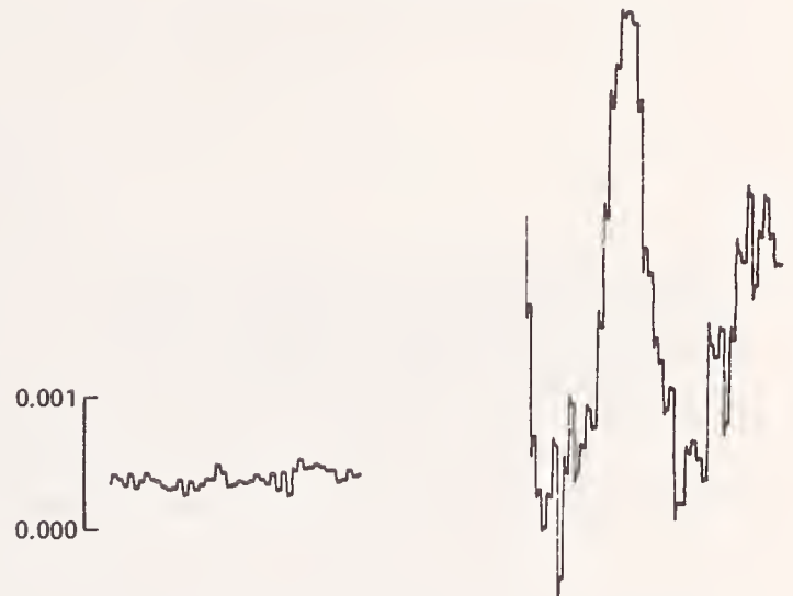
Figure 6. OFT trace of the scattering from the #20 standard scratch at 0.6328 \mu\text{m} . The scale on the left is the same as in figure 5. The trace on the right was generated using a factor of 100 increase in gain in the detector electronics. This figure illustrates the sensitivity of the OFT to extremely low levels of scattered light.
