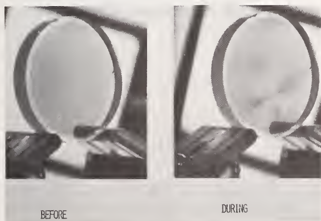
Figure 8. Coated KCl viewed through polarizer/analyzer before and during irradiation by 500 watts into a 1 mm spot size.
