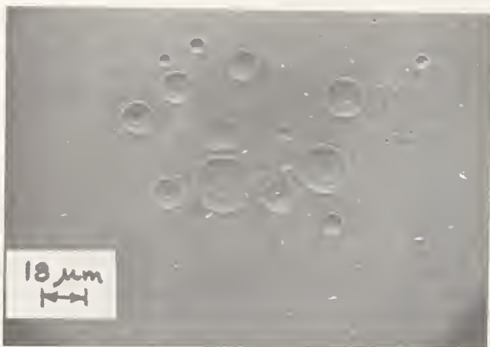
Figure 7. SEM photograph of a large damage site on rutile surface; the spot-size is 160 \mu\text{m} . Note that this is a single shot damage site and the small craters are irregularly distributed.
