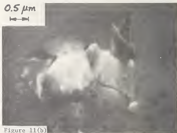
Figure 11. (a) SEM photograph of a large damage site on \text{YVO}_4 surface; a spark was observed and the spot-size is 160 \mu\text{m} . (b) Close-up view shows that the damage is due to a nonmetallic inclusion, 1.2 \mu\text{m} in diameter, which was about 0.2 \mu\text{m} below the plane surface. The morphology has crack nucleation similar to that in reference 8.
