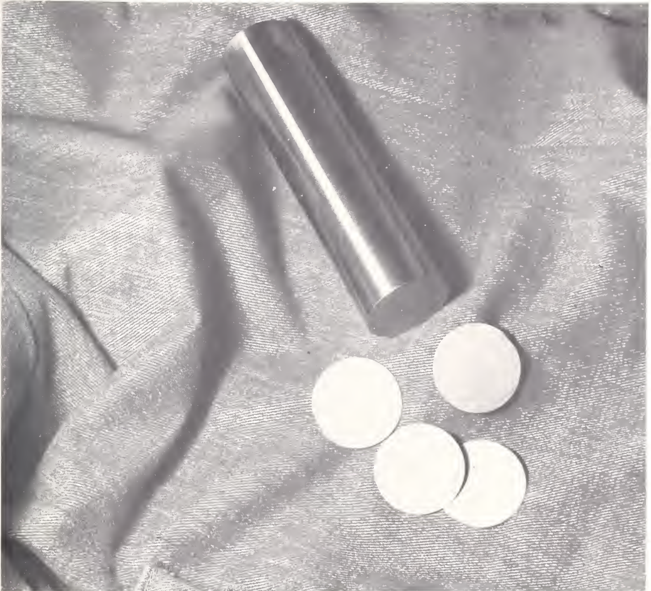
Fig. 15 The starting material for integrated circuits: a single-crystal ingot of high-purity silicon, and slices.
