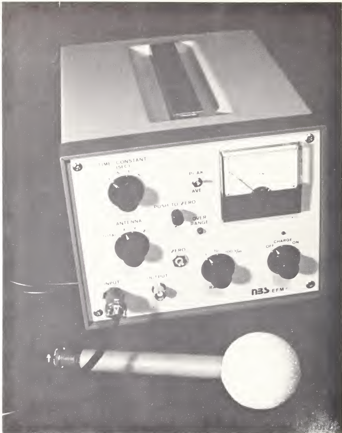
Fig. 75 The NBS EFM-5 probe package. A significant feature of this instrument is that it provides coverage of the radio and television broadcast bands.
