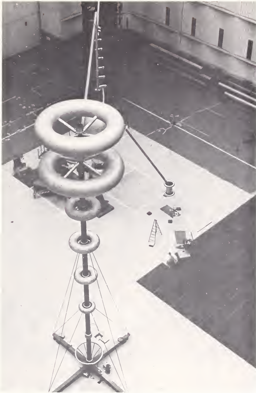
Fig. 65 NBS measurement of a very-high-voltage device in a French laboratory. The NBS apparatus appears as a small spool-shaped object at the center right of the photograph. Note the size of the stepladder and the person at the equipment rack.
