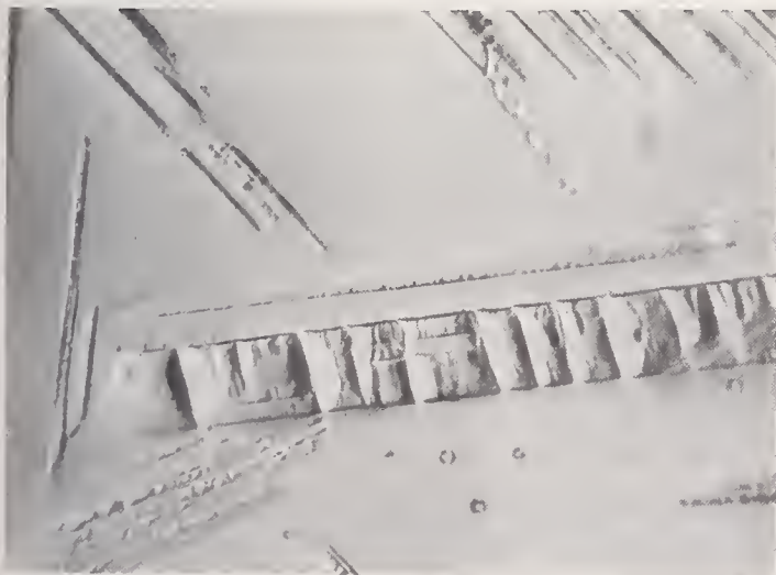
Martensite band produced spontaneously on cooling an unstable AISI 304 steel to 76 °K. The conversion of austenitic steels to martensite at low temperatures modifies their mechanical properties (page 123).
