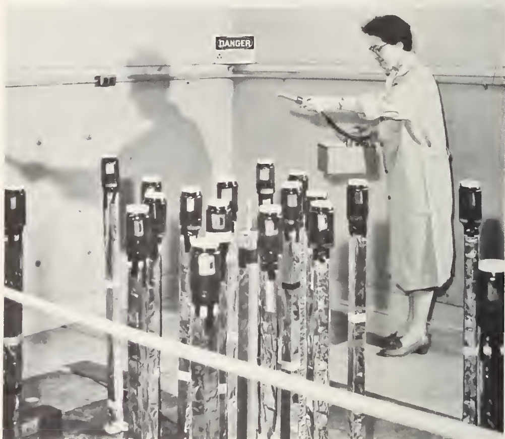
Surveying the radiation field around a calibrated cobalt-60 source (encapsulated in the lucite cylinder at the center) which is used to expose dental-size film packets. The film packets are ordinarily used to measure total radiation exposure of workers in hazardous areas (page 71).
