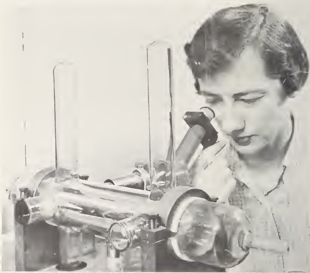
Vacuum microbalance used to determine the oxidation rate of niobium under various temperature and pressure conditions. Niobium has great potentialities as a high-temperature structural material. However its usefulness is at present restricted by its tendency to oxidize rapidly at temperatures as low as 450 °C (page 85).
