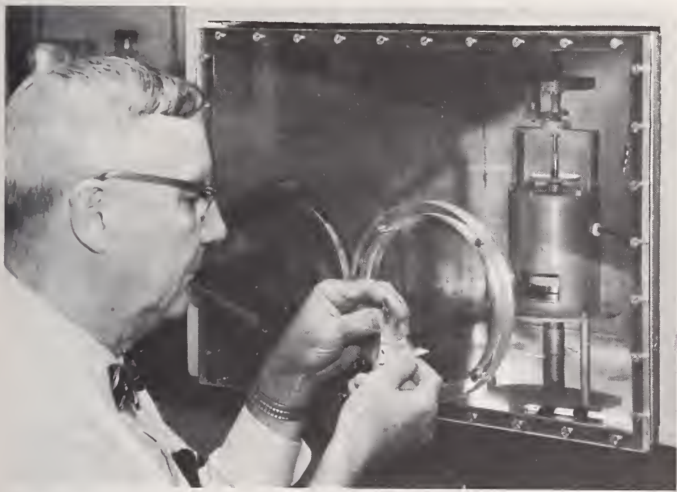
Dielectric reference materials are placed in constant humidity chambers for measurement of their electrical properties. The three-terminal guard-ring electrode holder recently developed at the Bureau for such work can be seen in the chamber (page 34).
