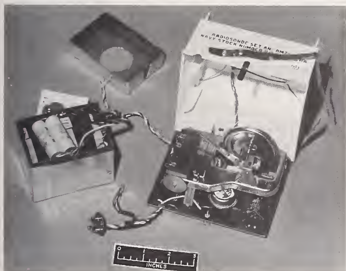
An improved transistorized circuit was developed for a radiosonde for telemetering upper-air meteorological information (page 103).
