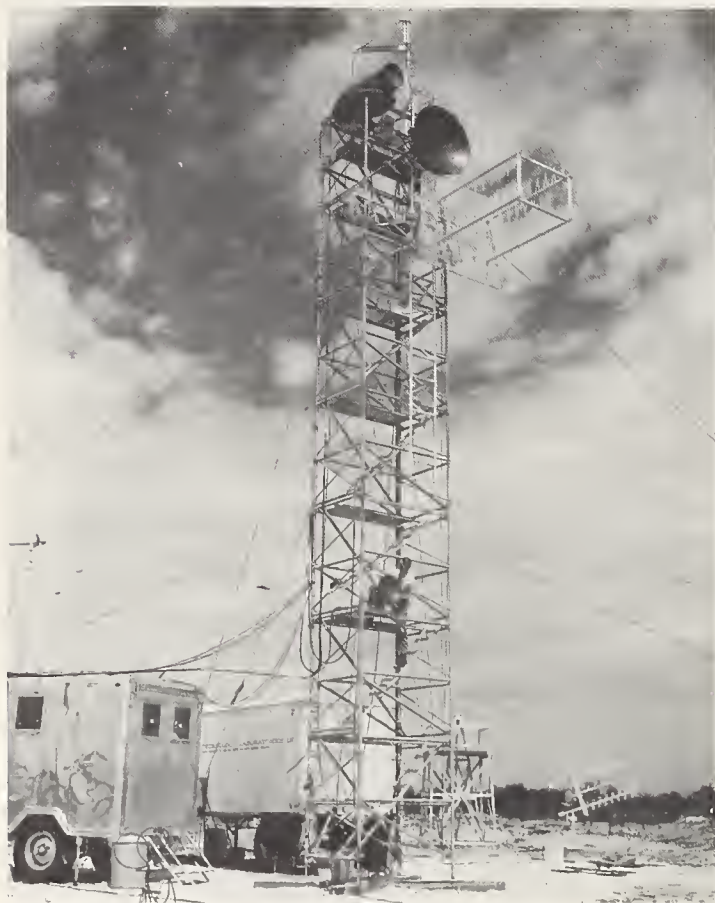
Equipment used to investigate the effect of atmospheric turbulence on radio direction finding and guidance systems. Measurements are made of the phase stability of radio signals propagated over line-of-sight paths (page 133).
