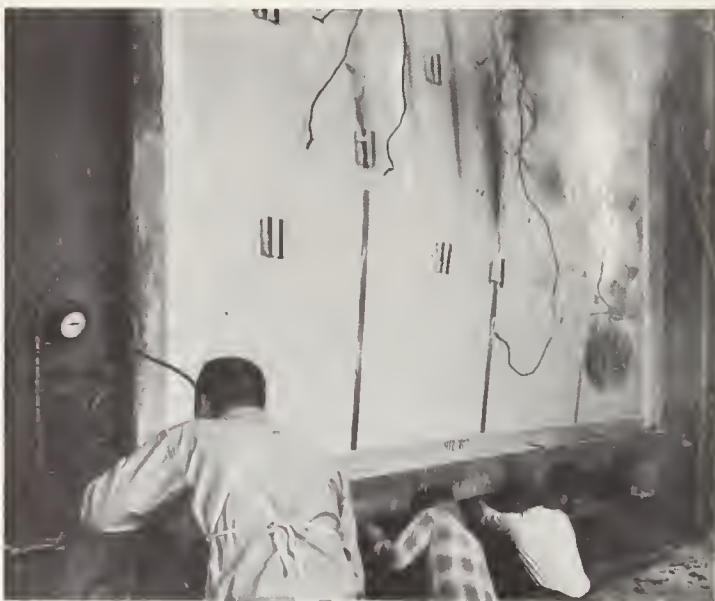
Prefabricated wall panel at the time of failure in a fire endurance test. The panel is of a special lightweight construction designed for use in arctic regions (page 109).
