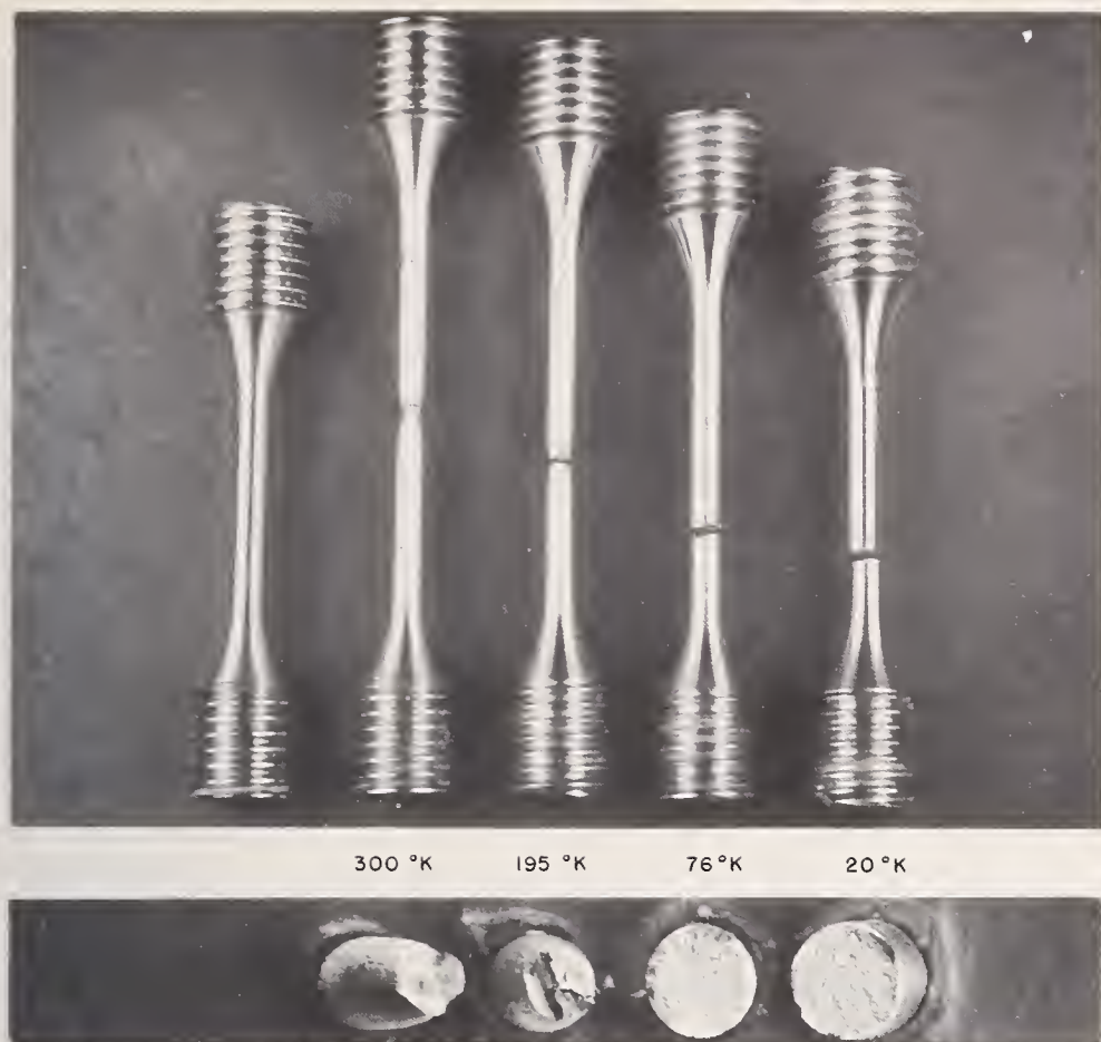
Specimens show how ductility of annealed AISI 202 steel decreases as its temperature is lowered. Unbroken specimen at left shows original size (page 123).
