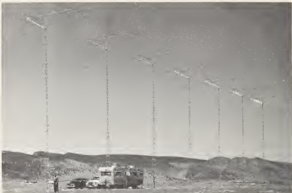
Seven 5-element Yagi antennas erected at the Bureau's Table Mesa (Colo.) field site. The antennas, in conjunction with an electronic scanning device, are used to pinpoint the direction of radio signals received from forward scatter transmission (page 137).
