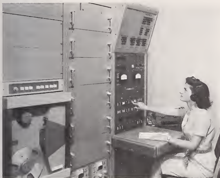
Special-purpose computer, AMOS IV, developed for the Weather Bureau for use as the central element in an automatic weather station. The computer collects and processes the data picked up by the station before it is transmitted (page 118).
