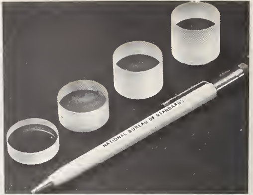
Thermal conductivity studies of small solid specimens using specially developed equipment. Specimens such as those shown at right have been studied at temperatures up to and above 800 °C (page 111).
