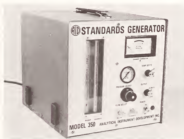
Figure 3. The Model 350 Standards Generator showing the gas flowmeters and temperature readout.
