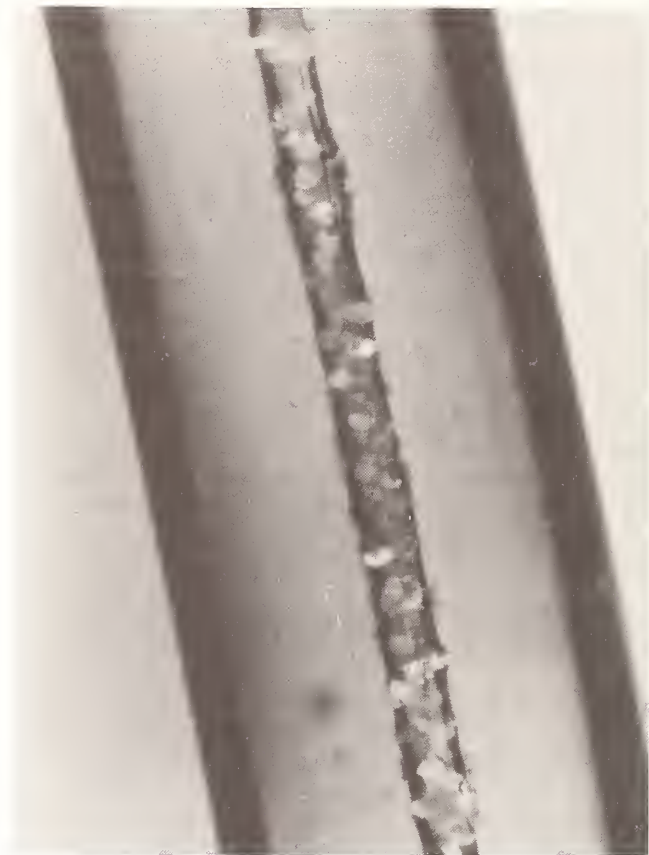
Figure 7. Microphotograph of a section of alumina-packed microcapillary (75 \mu\text{m} , i.d.) for liquid chromatography. Reproduced from T. Tsuda and M. Novotny, Anal. Chem. 50 , 271 (1978).
