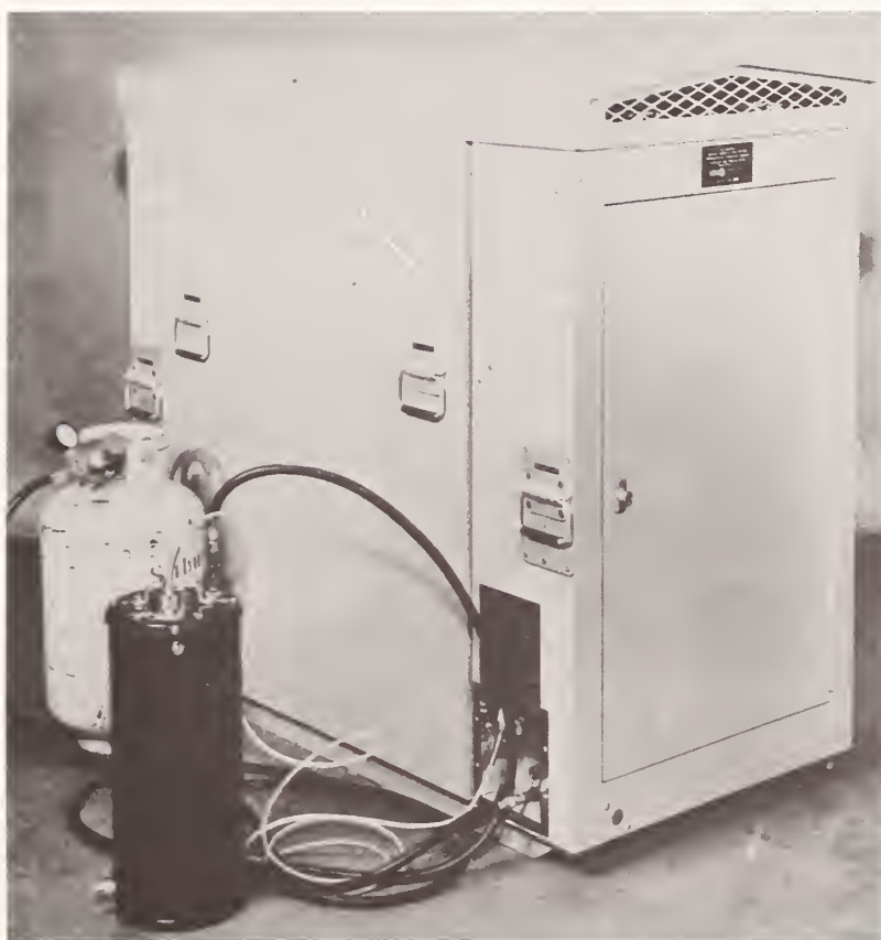
Figure 7. Automatic sampler, closed and secured; dimensions are 134 \times 69 \times 130 cm. Pump is in its black container.
