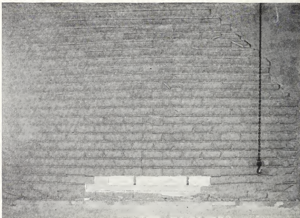
FIGURE 5. Exposed side of partition 9 showing the hole that limited the fire resistance of the partition.
