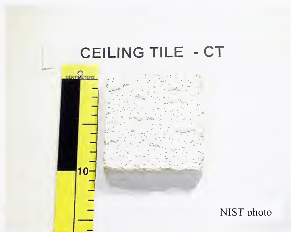
Figure D-16. Photograph of Acoustical Tile Showing Factory Painted Surface.
