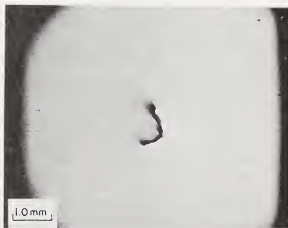
Figure 8. Electron beam induced images of a "bare" (111) oriented, 150 \Omega -cm, p-type silicon wafer which has been mechanically polished. a) analog of the surface photovoltage image showing residual polishing damage on the wafer. b) conventional secondary electron image of the same area of the sample showing the topography of the surface.
