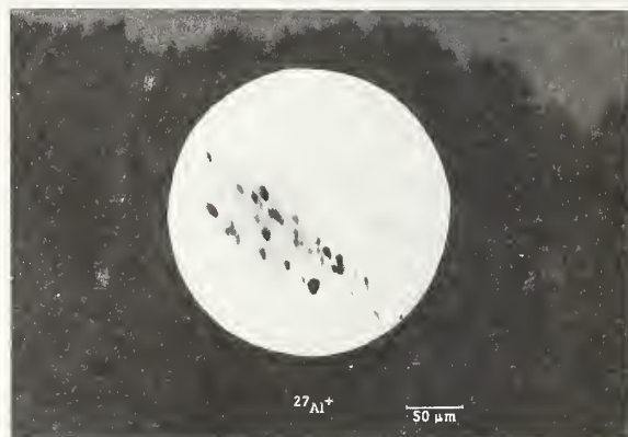
Figure 23. Aluminum ion image of platinum - aluminum thin film sputtered onto silicon at Al/Si interface.
