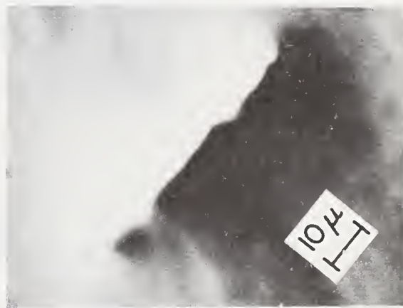
Figure 13. Scanned surface photovoltage image of a defect, apparently a microsplit, which was introduced during saw cutting of the (100) surface. The microsplit is thought to be flanked by stacking fault arrays in the \langle 110 \rangle direction on the surface.
