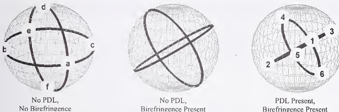
Figure 3: Simplified representation of the polarization state trajectories associated with the 6-state generalization of the M/S technique for both the measurement system and DUT.
