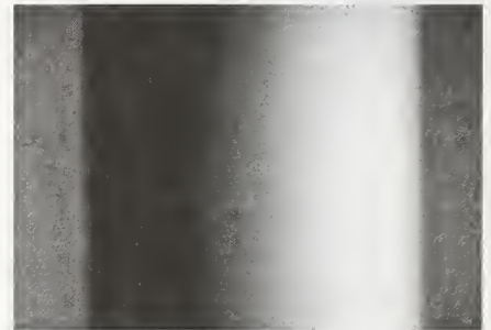
Figure 4: Birefringence image of an optical fiber bent through a radius of curvature of 1cm. The center of curvature is to the left. Image size 176 × 121 \mu\text{m} .
