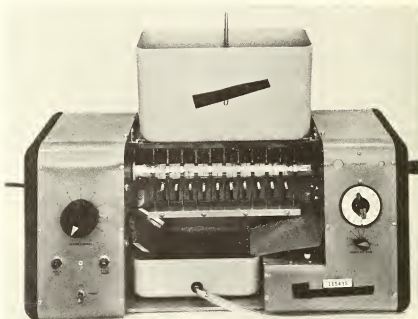
Figure 16. Multiple zone apparatus used for the purification of organic materials.
