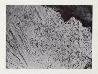
Figure 1. Micrograph of the heavily etched alloy wire.
