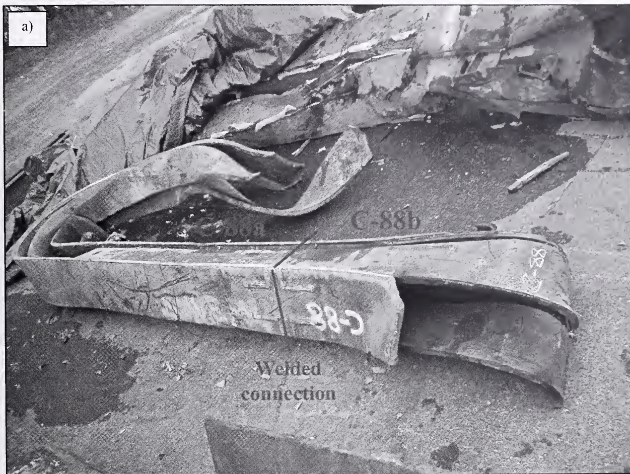
Figure 3–13. Core columns recovered from WTC 2. a) C-88a (801B: 80–83), lower 16 ft of built-up box column and C-88b (801B: 77–80), upper 8 ft of built-up box column.
