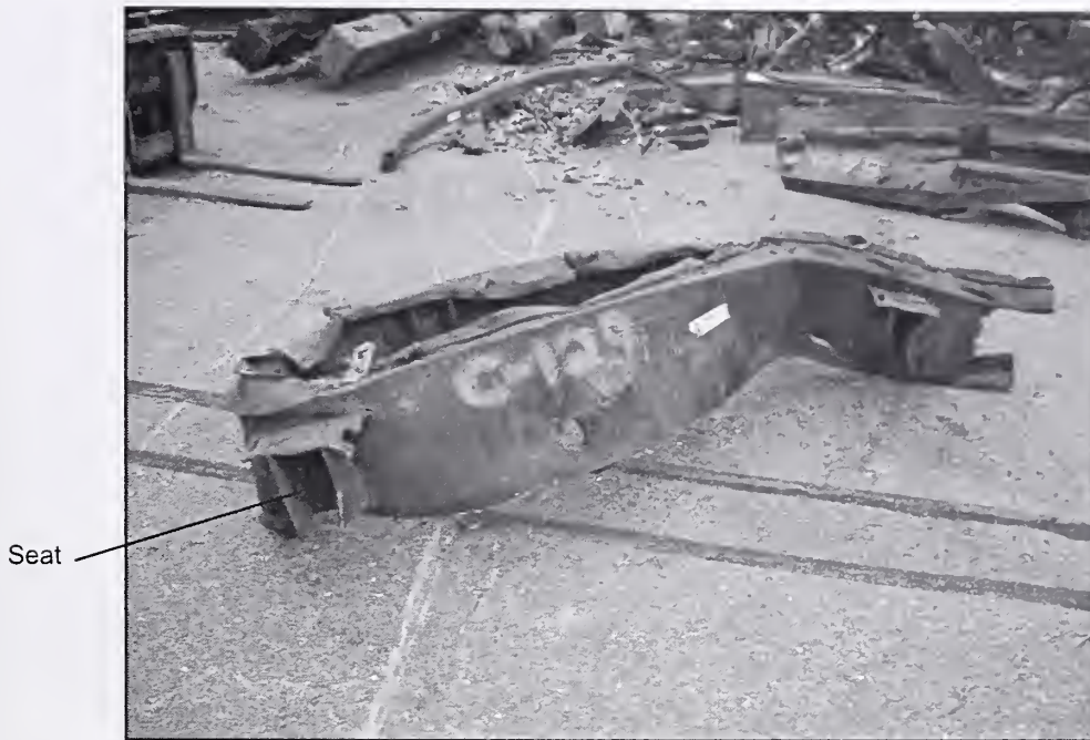
Figure A-11. Recovered inner channel material used to connect floor trusses to core columns; shown is sample C-129.
