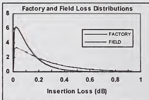
Figure 5. Insertion loss distributions for factory and field (random) connections.
