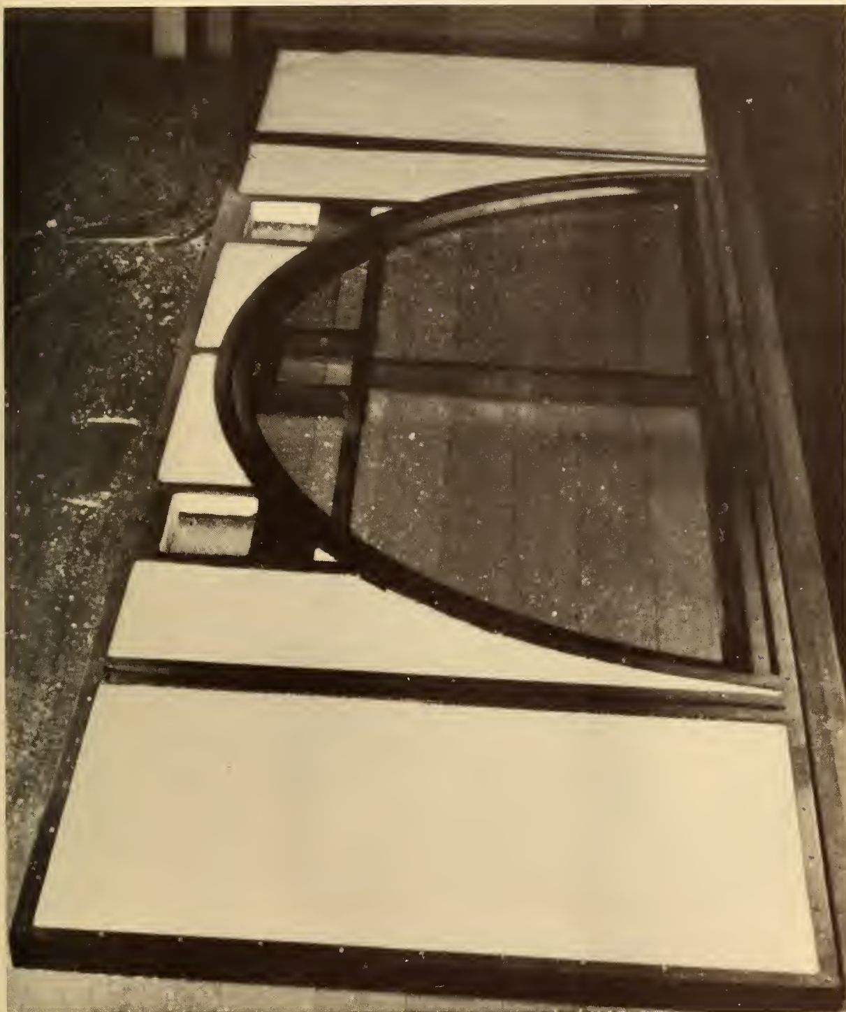
FIGURE 3. 35°C BATH COVER WITH ONE SIDE REMOVED TO SHOW POLYSTYRENE FOAM FILLER
