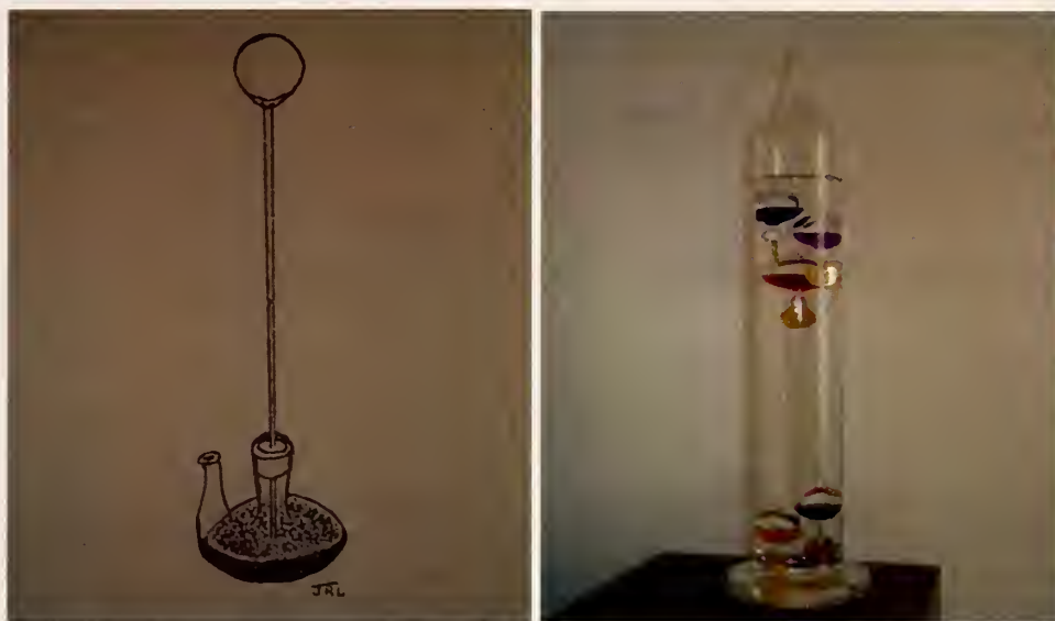
Figure 1 Galileo thermoscope sketch (left) photograph of modern thermoscope (right).
