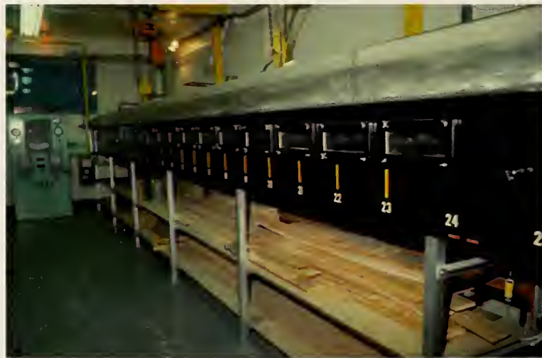
Figure 3 Photograph of Tunnel Test Apparatus, ASTM E84, NFPA 255, & UL 723
