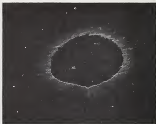
Figure 10. Scanning electron microscope (SEM) photograph of a damage site produced by a Q-switched pulse. The site dimension is 250\ \mu\text{m} from left to right.
