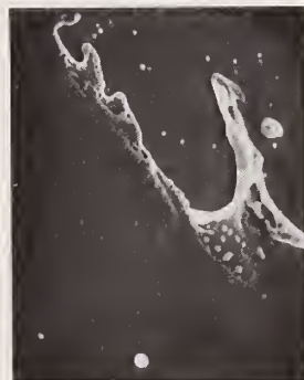
Figure 72. High magnification SEM picture of the extreme edge of the area. Molten ZnS films and cracked ThF 4 films can be clearly seen.
