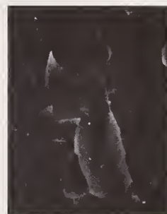
Figure 45. Detail of stress disruption. This characteristic is typical of the 100 percent \text{ZnS} films.
