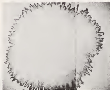
Figure 43. Low magnification picture of a moderate to heavy damage site. The typical light damage annulus surrounds the main, heavy damage area.
