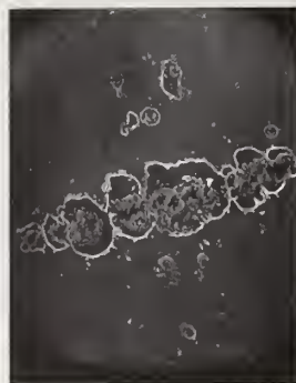
Figure 55. This is a view of damage sites which clearly indicates a crater type of delamination in the film.
