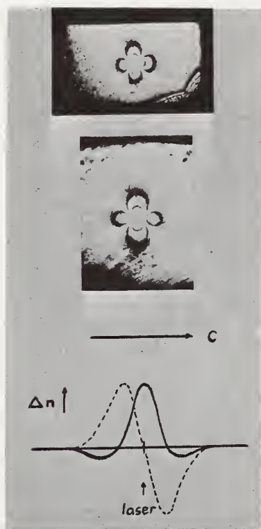
Figure 8. Typical laser induced birefringence patterns in \text{LiTaO}_3:\text{Fe} (0.05%). The line drawing is a plot of the birefringence change along the c axis. The broken line is the birefringence change which would occur due to space charge fields due to diffused carriers.
