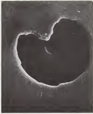
Figure 34. Detail of a removal site. A nucleus is evident but no evidence of fused material.
