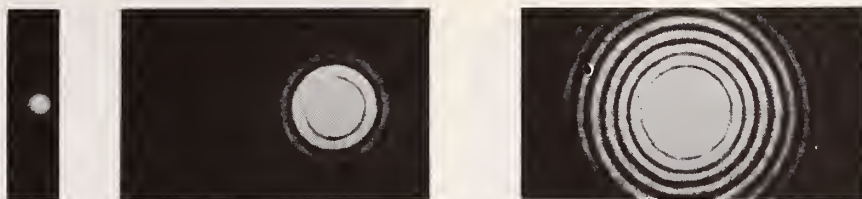
Figure 3. Photographs of the diffraction pattern of the giant-pulse ruby laser oscillator (Fresnel No. 0.4) at 3 Rayleigh distances (far field) from the laser. The three photographs were exposed under three different beam attenuations.
