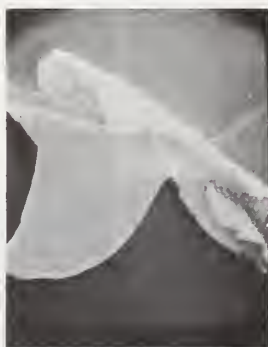
Figure 89. Perfect illustration of shear of the PIHF due to damage occurrence at a lower level. The curling of the film demonstrates its tensile property clearly indicating that it is mostly \text{ThF}_4 .
