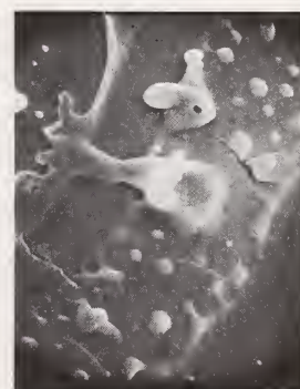
Figure 63. Picture shows distinct evidence of at least one film having been completely fused causing cracks in the adjacent films. The molten film or films are presumably the much weaker ZnS films. The Thorium Fluoride films are cracked and split. Outer 3 films only are affected.
