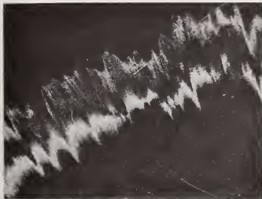
Figure 3. Section of damage ring near threshold 100X magnification.
