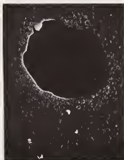
Figure 19. High magnification SEM picture of a removal area. The partially damaged film surrounding it shows a peculiar but uniform texture. Note the absence of fused materials around the removal site.
