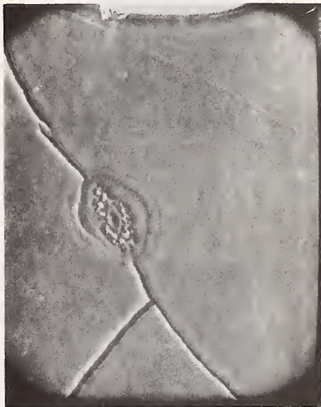
Figure 74. This high magnification picture clearly shows the nature of one of the nucleus/crack systems observed above. The nucleus is in fact a very small crater with smooth walls rather than the 'stepped walls' observed in multilayer structures. The remarkable feature of the crack is that it does not penetrate the whole thickness of the film and appears to extend only to the point where thermal failure occurred.
