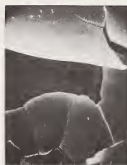
Figure 31. High magnification of a mechanically damaged area the columnar growth pattern of the film can be clearly seen.
