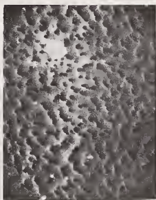
Figure 42. Granular damage in the same area. Spacial frequency of the small pits is higher than in the VPM 5 samples.
