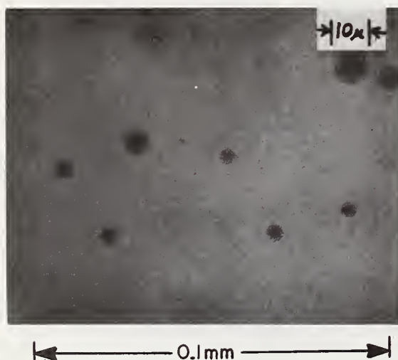
Figure 10. Laser-induced damage occurring before a detectable spark in a single quarter-wave film of \text{TiO}_2 .
