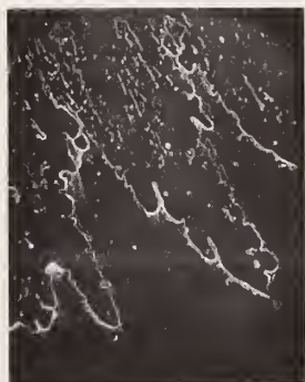
Figure 71. Low magnification SEM picture of the above area; the ejected molten material is clearly shown.
