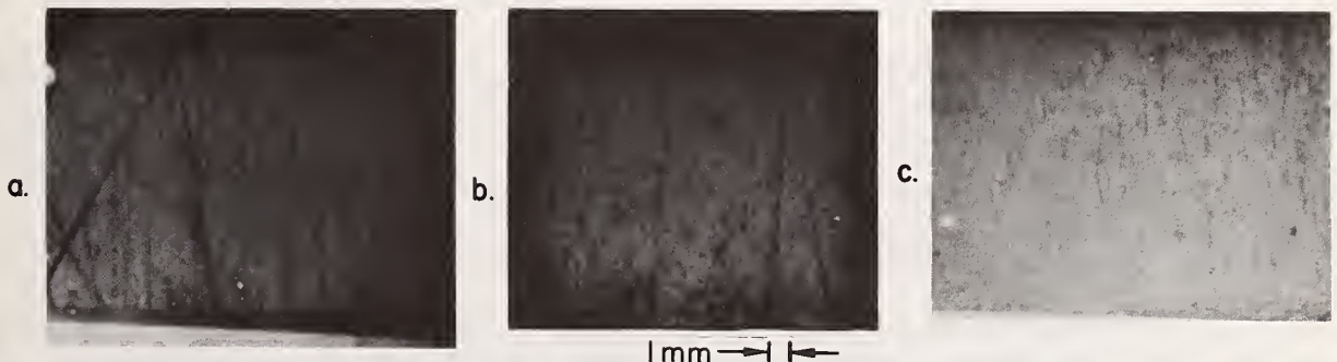
Figure 2. Examples of x-ray diffraction topographs taken for (a) abrasively polished sample, (b) \text{Ar}^+ ion polished for 2 hours ( 7\text{kV} @ 300 \mu\text{A}/\text{cm}^2 ), (c) same conditions as (b), but for 4 hours.
