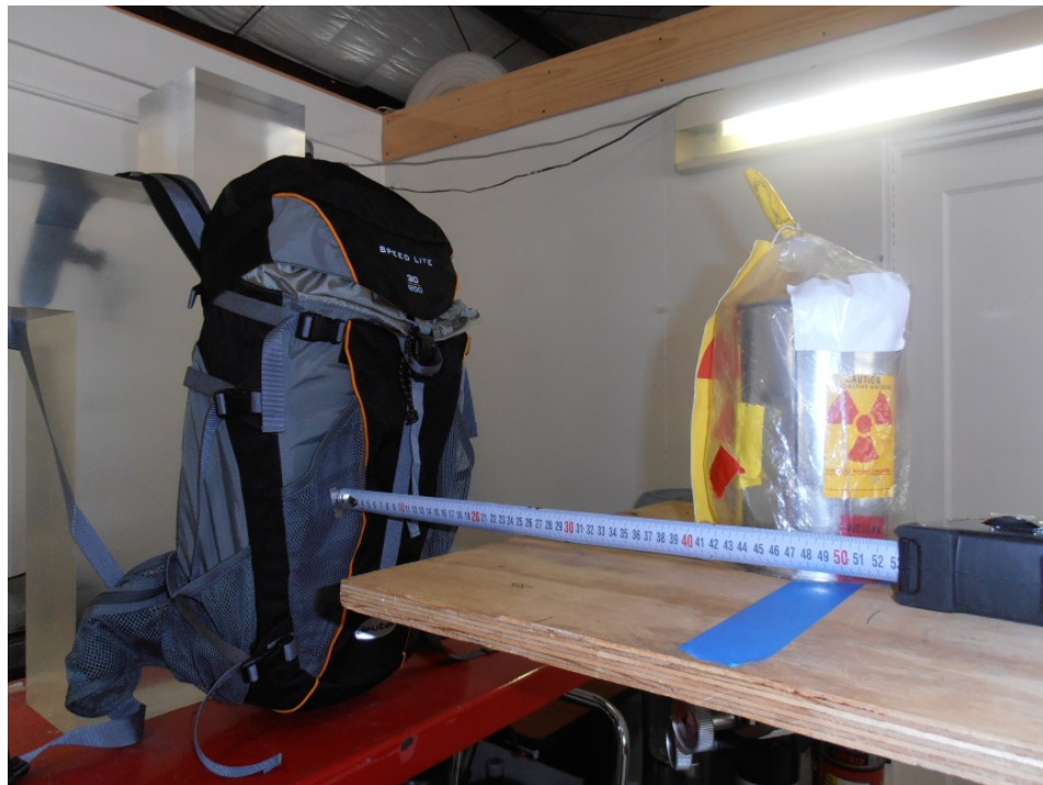
Figure 2: BRD mounting on phantom and source location relative to BRD
