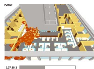
Computer animation showing flame iso-surface in office suite at 7 min 30 s after flaming ignition.
