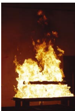
2.0 MW heptane fire from liquid spray burner.
