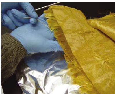
Extraction of yarns from body armor panel for chemical and mechanical analysis.
