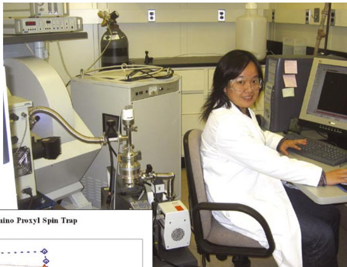
A BFRL researcher uses the electron paramagnetic resonance (EPR) spectrometer to determine the generation of free radicals in titanium dioxide ( \text{TiO}_2 ) suspensions; inset shows EPR data, concentration changes of the nitroxide free radical traps, 3-amino proxyl (AP) as a function of UV irradiation time for a series of \text{TiO}_2 materials.
