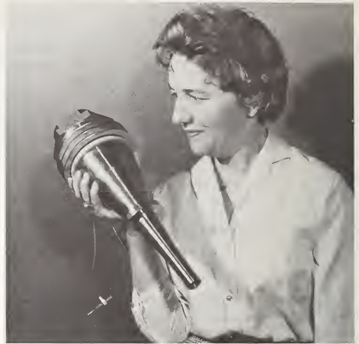
FIGURE 2. Fifteen horsepower sonic motor with catenoidal full wave horn design.
