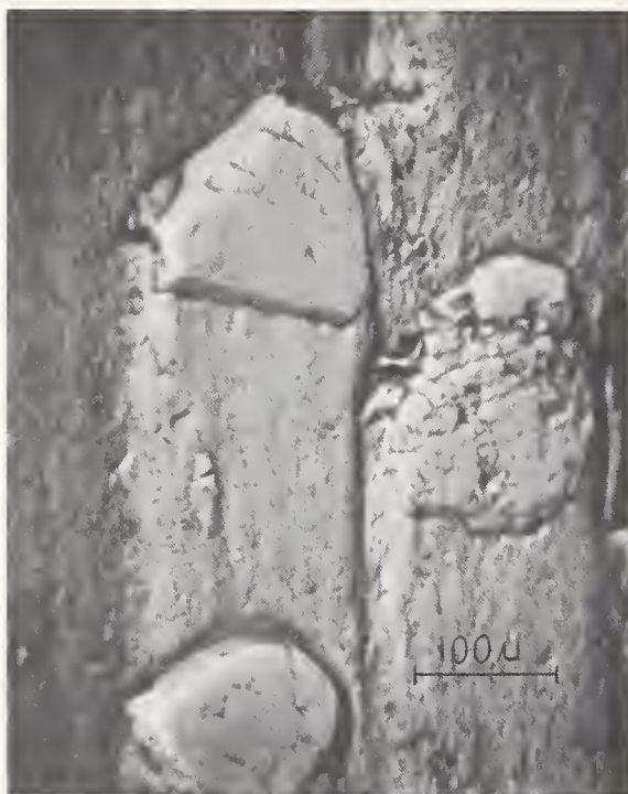
FIGURE 14. Scanning electron micrograph of a replica of the metal bond wheel containing 80/100 DXDA.
