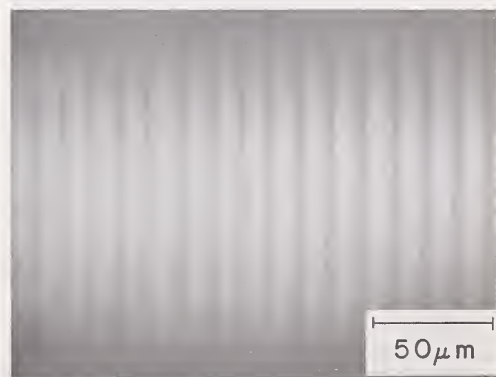
FIGURE 7. The surface of a sapphire rod flame-polished under ideal conditions in this work.
