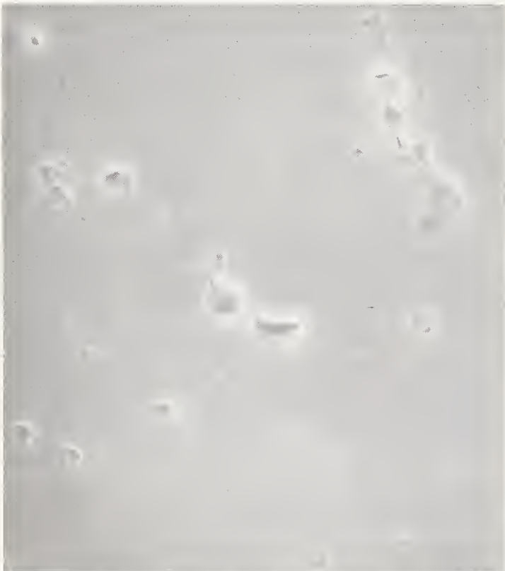
FIGURE 4. Precision polished substrate from same lot of 99.5 percent alumina as in fig. 2 and 3. 1000x, showing open pocks (SEM).
