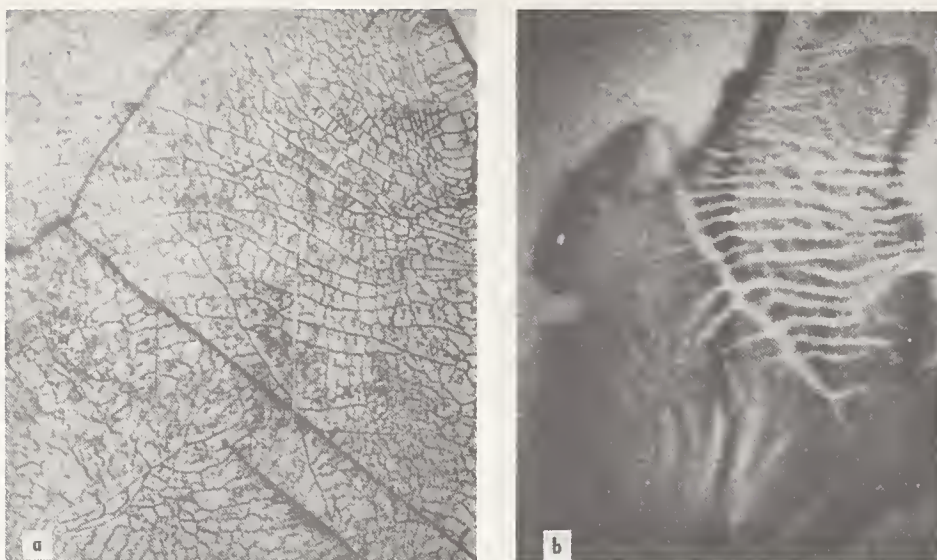
FIGURE 12. (a) Single crystal of ZrC etched on a (100) plane in 1:1 boiling H_2SO_4 to show both individual dislocations and dislocation of sub-boundaries, 9X. (b) X-ray image of same area as in (a) showing the boundaries to be of a tilt character, 5X.
