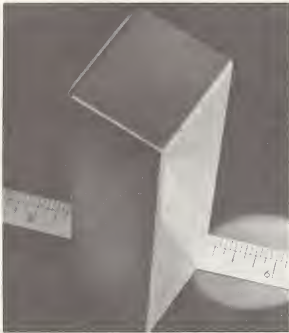
FIGURE 3. 96 percent alumina rectangle ground to a reflective surface with a roughness of 0.08 \mu .
