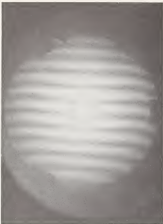
FIGURE 15. The fringe pattern, observed with an interferometer, from a paraboloid produced by ion-beam figuring. From Ref. [11].
