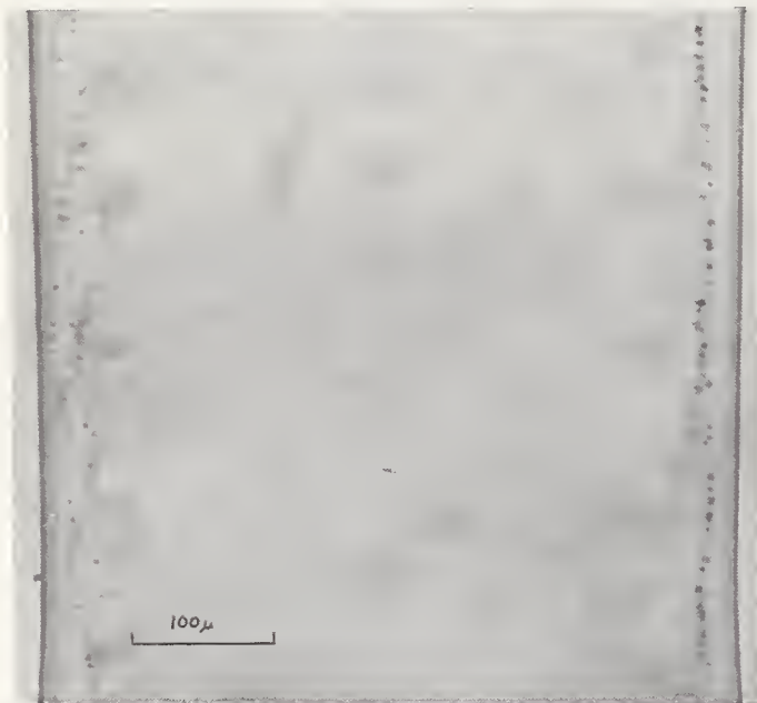
FIGURE 5. Photomicrograph of slightly overpolished filament showing that the necked-down region has not penetrated the void layers. Mid-plane section.
