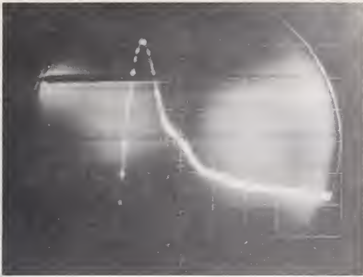
FIGURE 3. Oscilloscope showing the duration of a light pulse. Time scale: 1 \mu\text{s}/\text{div} .
