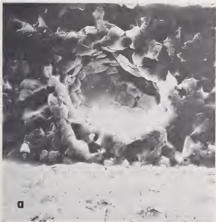
FIGURE 4. SEM pictures of surface void observed on a ground and annealed isostatic pressed substrate with a fine line test pattern present. The smooth equiaxed grain structure within the void indicates formation prior to or during sintering. (A) 1000X (B) 5000X.
