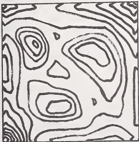
FIGURE 7. Drawing of typical Moiré line pattern on a 1000-line grid formed by a 2 in \times 2 in as-fired substrate showing combined flatness and waviness of about 0.004 in. (Each line corresponds to a contour interval of about 0.0005 in.)
