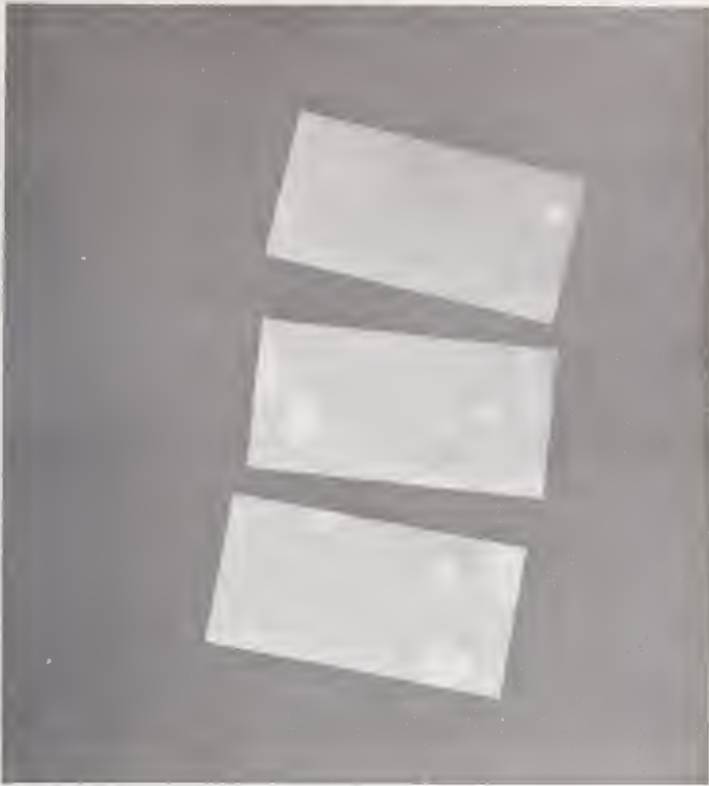
FIGURE 1. Non-homogenous structure in 1 in \times 2 in substrate of 99.5 percent alumina; lighter areas show about 1 \mu in roughness, while darker areas are 6 to 12 \mu in, pattern is full thickness of 0.0B5 substrate.
