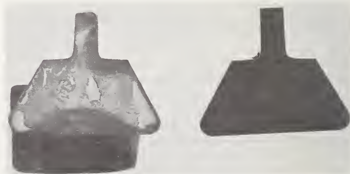
FIGURE 15. Template cutting tools, new and 3 hours wear.
