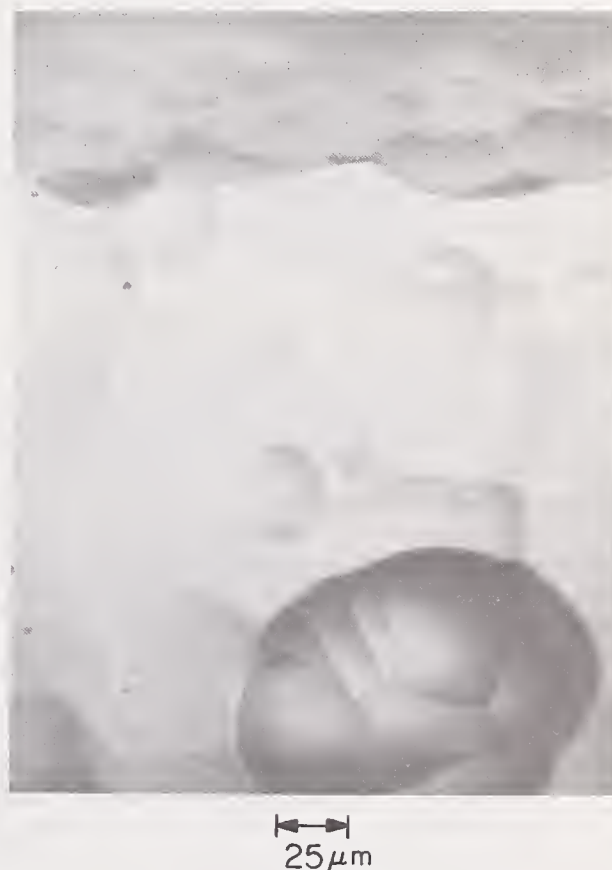
FIGURE 8. RF sputtering of specimen edge. Top of photograph is looking down the edge of an Al 2 O 3 rich MgAl 2 O 4 crystal specimen. The edge was rounded prior to polishing, then the specimen was sputtered approximately 54 hours.
