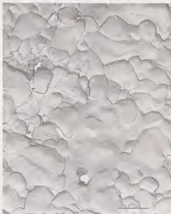
FIGURE 6. Electron photomicrograph—as-received surface, pressed, green machined and fired. Fiducial bar equals 5.0 microns.
