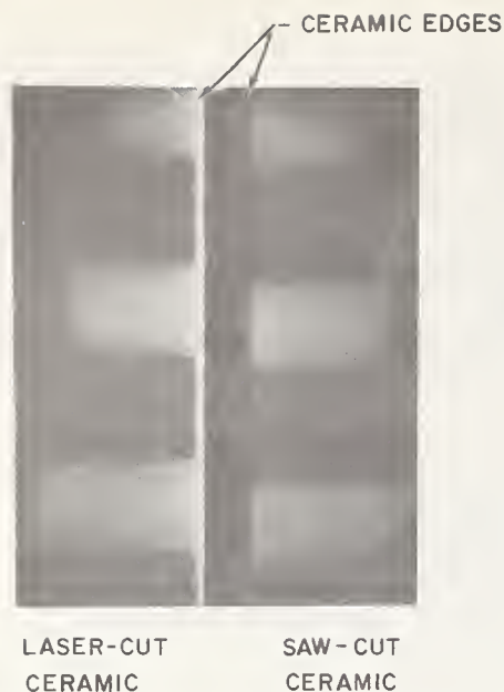
FIGURE 2. Zyglo test on laser-cut and saw-cut ceramic substrates.
