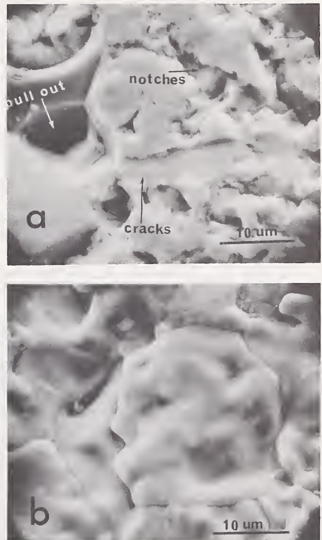
FIGURE 3. Scanning electron micrographs showing diamond cut surface of Al 2 O 3 prior to heat treatment (a) and after heat treatment (b). Heat treatment was 50h at 1700 °C.
