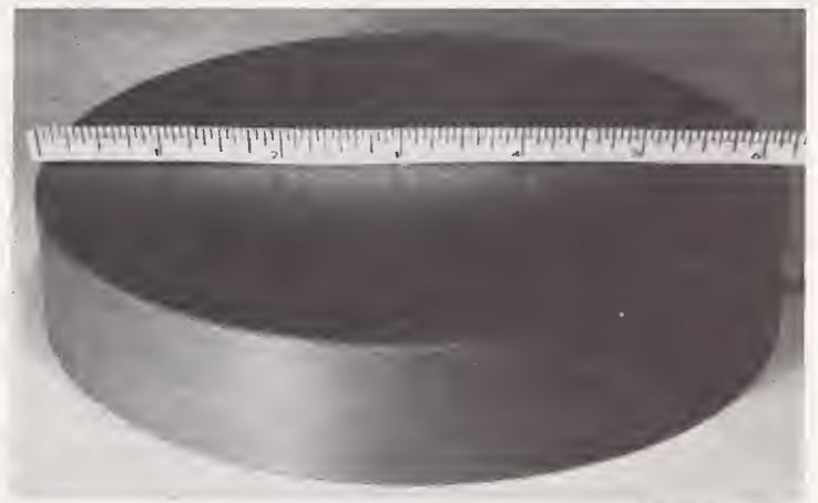
FIGURE 2. 96 percent Alumina disc. Ground to a reflective surface with a roughness of 0.08 \mu .
