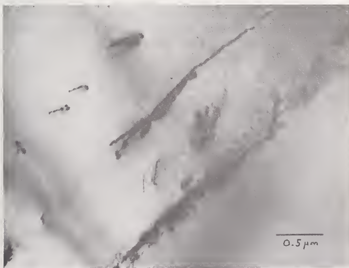
FIGURE 8. Basal microtwins produced within surface grain of polycrystalline aluminum oxide by diamond-grinding.
