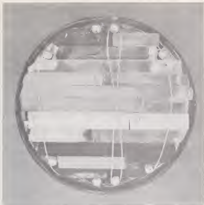
FIGURE 2. RF sputtering holder. Note ceramic bars held in place by wires.
