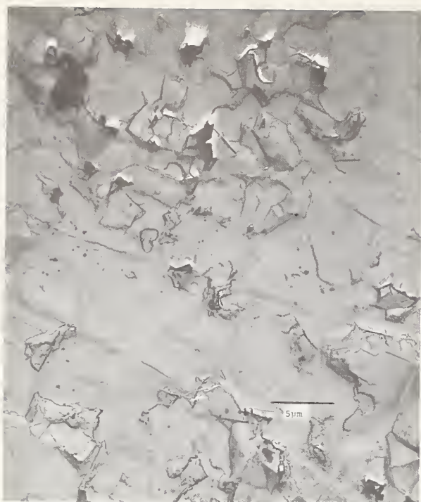
FIGURE 8. Standard shop grind plus lapping with 15, 7, 1 and 1/4 micron diamond.
