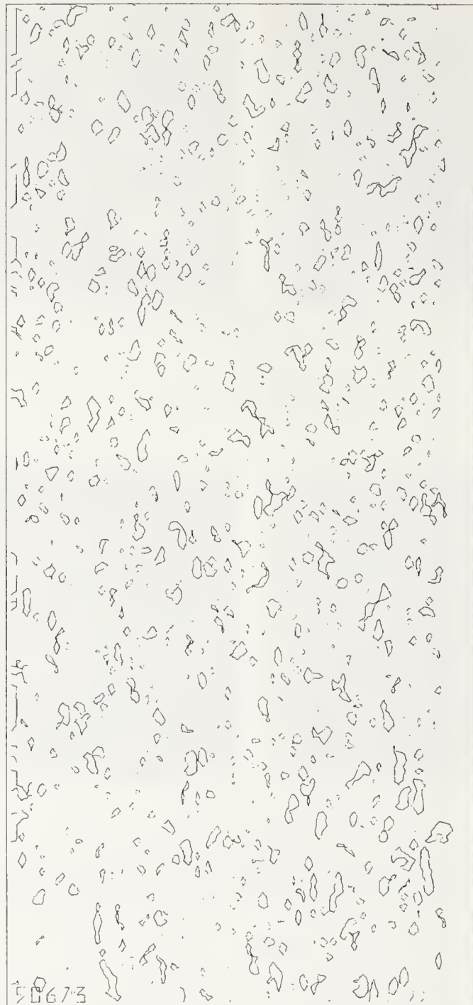
FIGURE 11. Profilometer image of Novaculite surface. The rastered profilometer image contoured at a 50 percent level by computer processing. Multiple contouring would give a topographic map of the surface.
