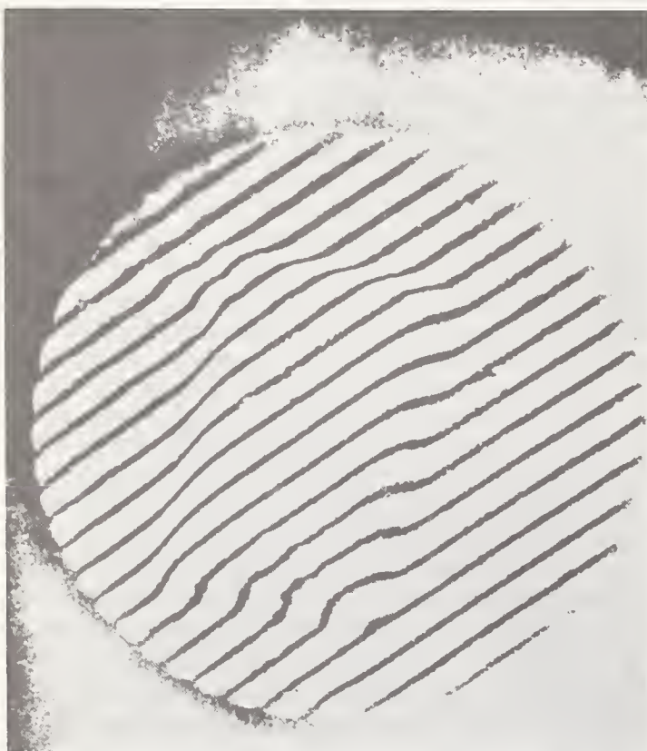
FIGURE 1. Interferogram showing uniform removal in a rectangular pattern.
