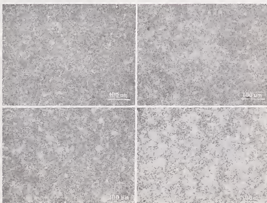
FIGURE 6. Surface textures of tape-cast 99.5 percent alumina substrates from different lots shipped by same supplier.
