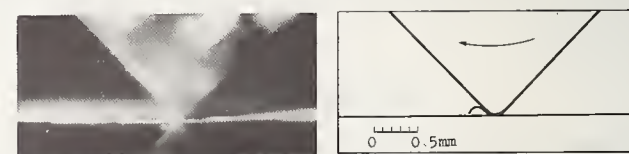
FIGURE 11. Chip from hardened steel. Photographed at the position "c" in figure 4. U=12.5 m/s, v=0.042 m/s.
