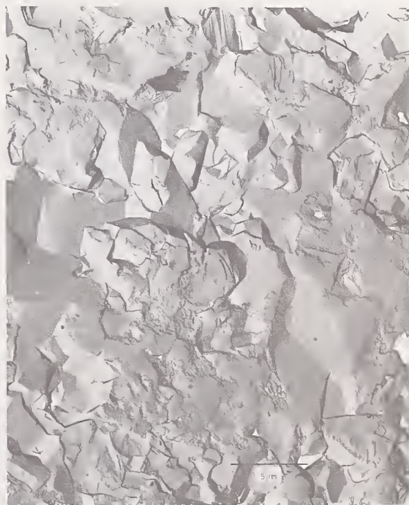
FIGURE 7. Electron photomicrograph—15 rms surface created by standard shop surface grinding. Fiducial bar equals 5.0 microns.
