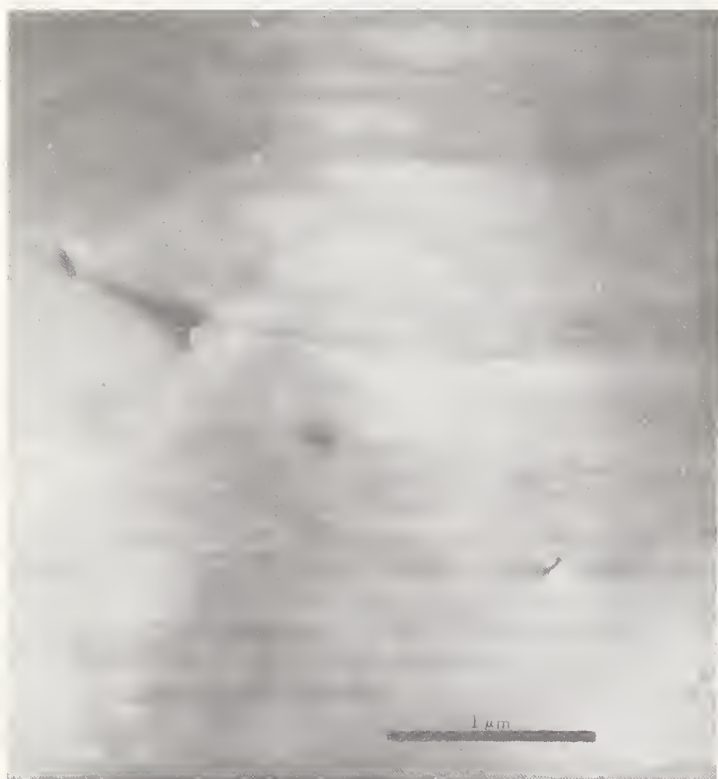
FIGURE 13. A row of dislocations which form a low angle boundary in an undeformed ZrC single crystal.
