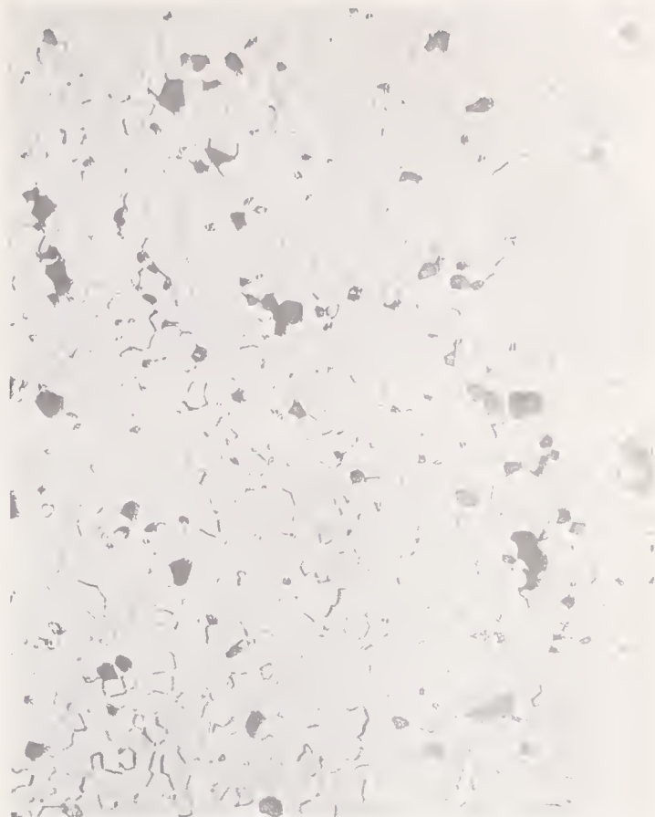
FIGURE 6. Hot pressed MgO fabricated with LiF additive. (150X)
