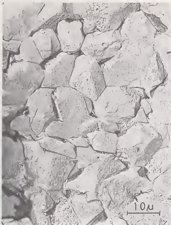
FIGURE 12. Electron micrograph of a replica of an etched 96 percent alumina surface after grinding with a metal bond wheel containing 140/170 SND-MB.
