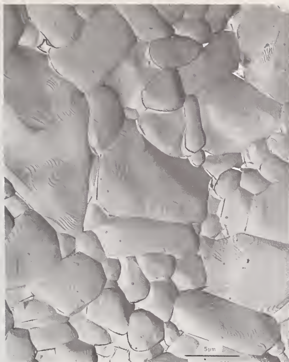
FIGURE 12. Electron photomicrograph—Surface produced by refiring a 15 rms ground surface in air. Fiducial bar equals 5.0 microns.
