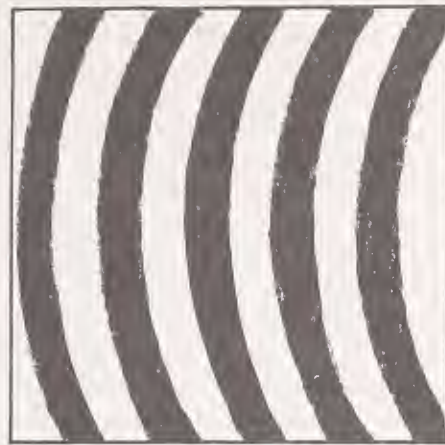
FIGURE 8. Drawing of typical Moiré line pattern on a 1000-line grid formed by a 2 in \times 2 in precision polished substrate showing absence of waviness and overall flatness of about 0.0002 in.
