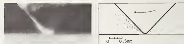
FIGURE 10. Chips from synthetic sapphire. Photographed at the position "c" in figure 4, U=12.5 m/s, v=0.042 m/s.
