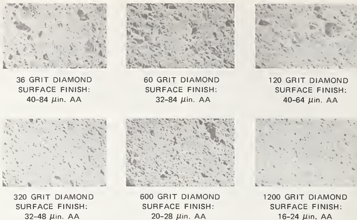
FIGURE 1. Scanning electron micrographs of Al-995 Alumina.
