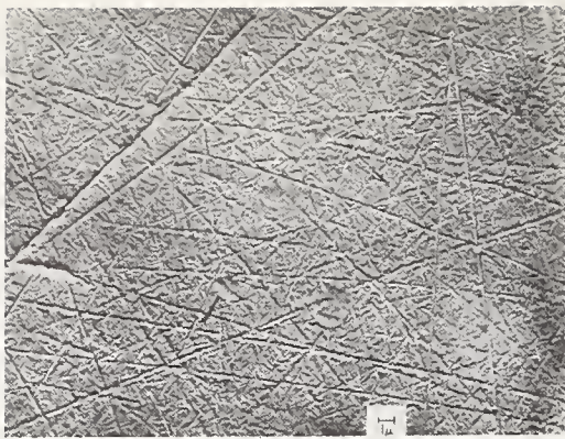
(A) 1/4 MICRON DIAMOND FINAL POLISH
