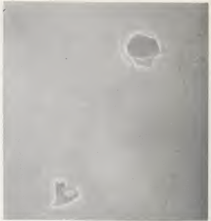
FIGURE 5. Precision polished substrate from same lot of 99.5 percent alumina as in fig. 2 and 3, 10,000x, showing fine line scratches from diamond polishing, most principal lines less than 0.00001 in wide, open pocks from inherent pores show intact wall detail, no "comet-tails" (SEM).
