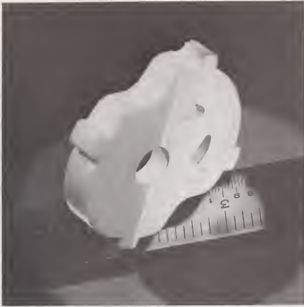
FIGURE 5. 96 Percent alumina ceramic valve disc ground to a finish of 0.15 \mu .
