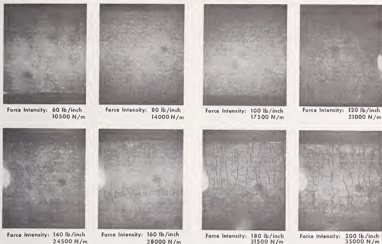
FIGURE 23. Workpieces ground under various force intensities for constant wheel sharpness.
