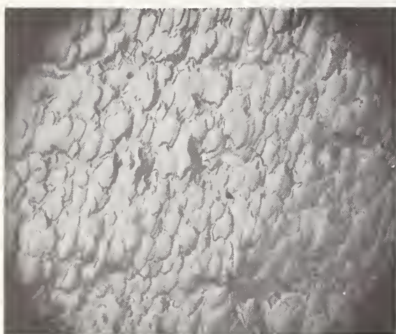
FIGURE 19. Ion beam sputtering of a medium grain (about 10–20 m) commercial \text{Al}_2\text{O}_3 (Alsimag 614). Electron micrograph showing elongation of depressions, exposed pores, and some traces of grain boundaries.
