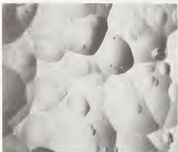
FIGURE 4. RF sputtering of ground spinel crystal. (A) as diamond ground (grinding direction vertical) (B) similar area of same specimen sputtered approximately 54 hours.
