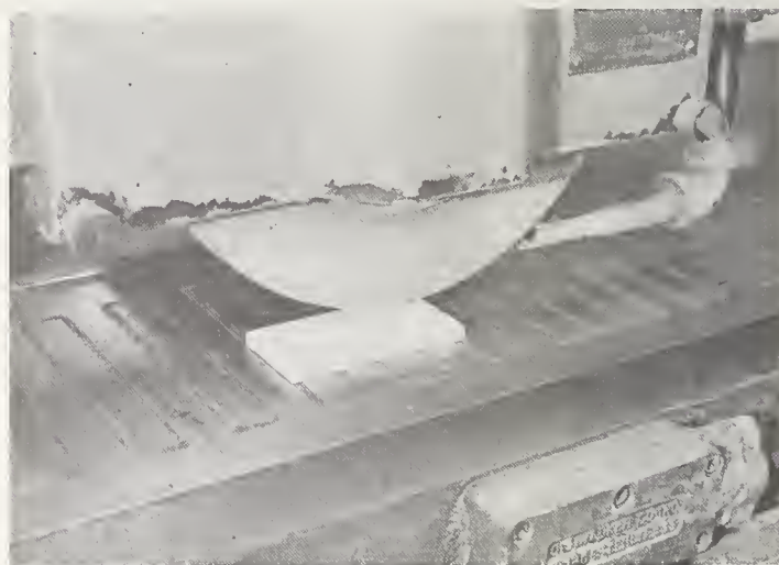
FIGURE 2. Grinding with specimen rotating as well as grinding wheel.
