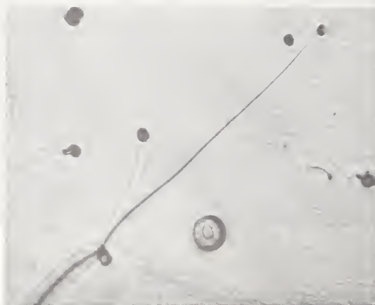
FIGURE 12. Craze pattern and cracks on RF sputtered soda lime glass.
