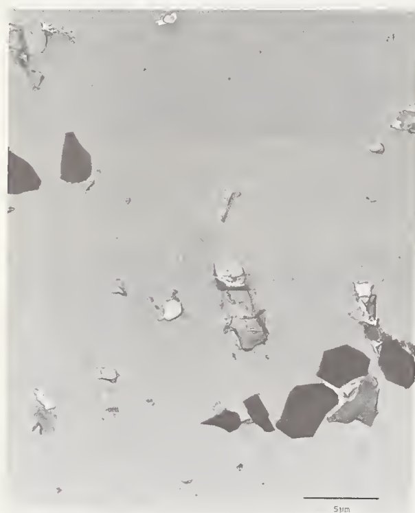
FIGURE 9. Electron photomicrograph—<1 rms surface developed using metallurgical laboratory lapping techniques. Fiducial bar equals 5.0 microns.
