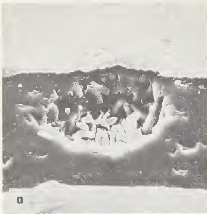
FIGURE 5. SEM pictures of surface void of a polished (unannealed) isostatic pressed substrate with test pattern present. The platelet structure within the void indicates the presence of foreign contamination. (A) 1000X. (B) 5000X.
