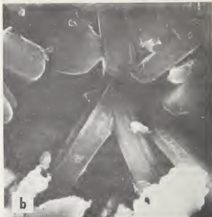
FIGURE 5. SEM pictures of surface void of a polished (unannealed) isostatic pressed substrate with test pattern present. The platelet structure within the void indicates the presence of foreign contamination. (A) 1000X. (B) 5000X.
