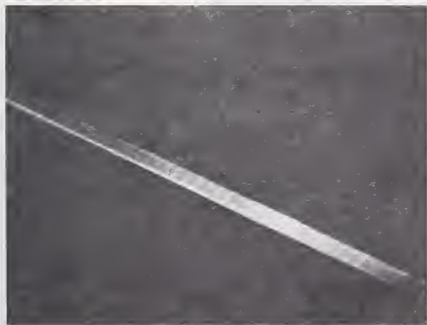
FIGURE 3. Optimum flame polishing conditions showing the stable molten sheath at the filament surface.
