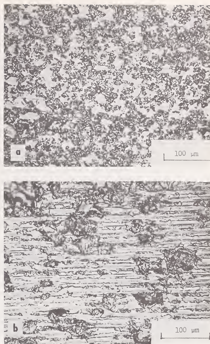
FIGURE 10. Photomicrographs of \{111\} surfaces of silicon single crystals ground in \langle 110 \rangle directions wet with a 46 grit alumina wheel at two rates of material removal. (a) d = 25.4\mu\text{m} , V = 0.042\text{ cm/s} (b) d = 25.4\mu\text{m} , V = 0.42\text{ cm/s} .
