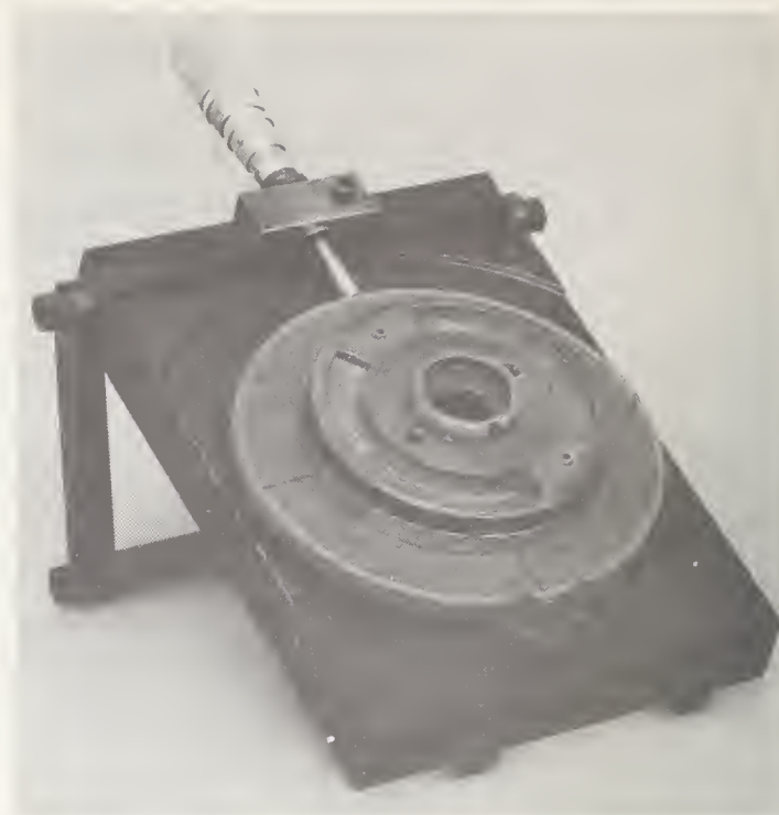
FIGURE 2. Special jig for measuring wear of wheels for surface grinding tests.
