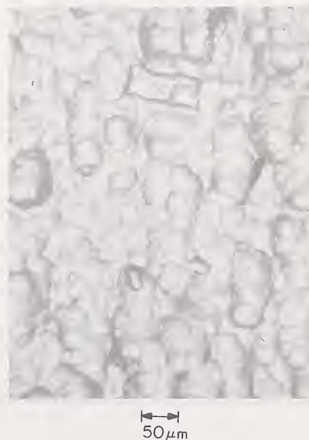
FIGURE 3. RF sputtering of ground surfaces. Ruby ground in vertical direction. Note remnants of grinding streaks. Note also the apparent imperfection revealed by sputtering (approximately rectangular object near top of photo).
