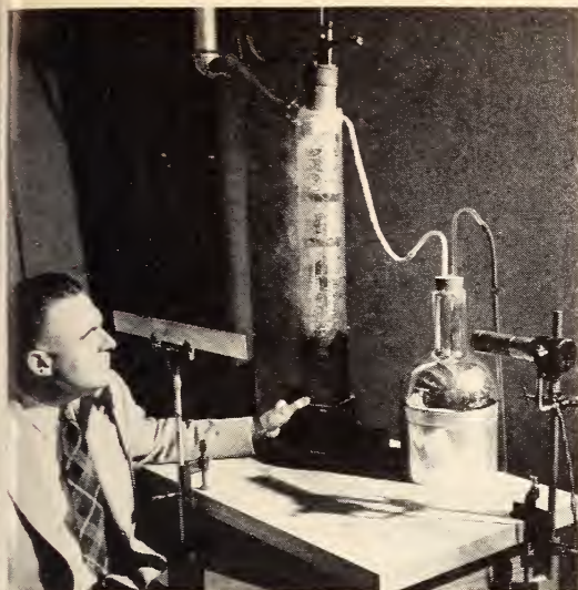
Left: Thermal Raleigh disk apparatus developed by NBS for the study of second sound and the properties of liquid helium II near absolute zero (p. 26). The new technique measures the torque exerted on a light disk (right) by standing waves of second sound set up within a resonant cavity.
