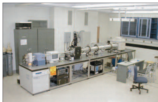
Figure 2. The world's first laboratory scale CD-SAXS prototype constructed on the NIST campus. Shown is the rotating anode molybdenum source (left side) used to generate high energy X-rays for transmission measurements on samples measured at varying angles of incidence on a 2-dimensional detector (back right).
