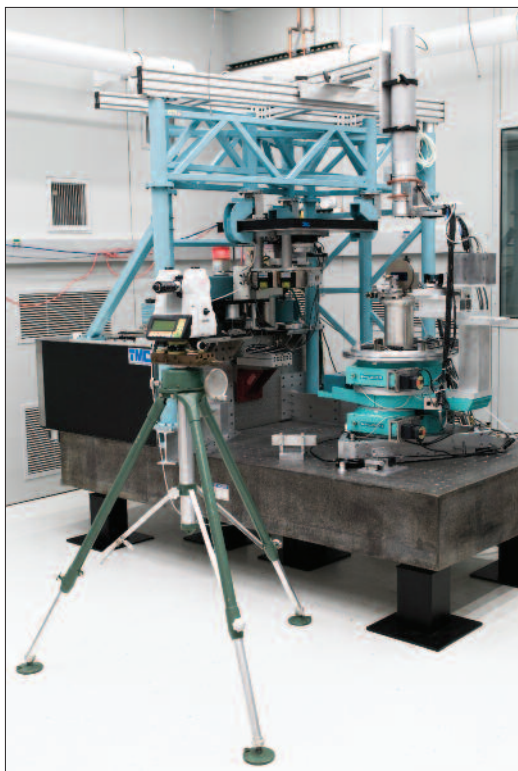
Figure 3. Ceramics Division Parallel Beam Diffractometer (CDPBD) located in the Advanced Measurement Laboratory at NIST seen during alignment of the new spherical air bearing under the goniometers (bottom of green goniometer stack). The X-ray source (near red light in center) is collimated through a monochromator (center, hanging from superstructure) and is diffracted/reflected by a section of a wafer (right) into an analyzer crystal and detector (right). Sample and Detector rotation axes must be coplanar with the incident and diffracted/refracted X-rays. This requires external optical alignment methods using autocollimation, e.g., by a Leika digital theodolite (front, left).
