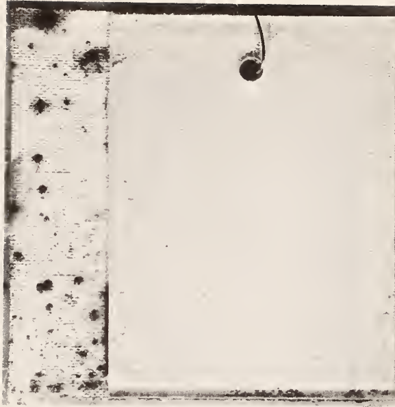
Figure 5. The backing material at the left has developed fungal growth during the fungus resistance test.
