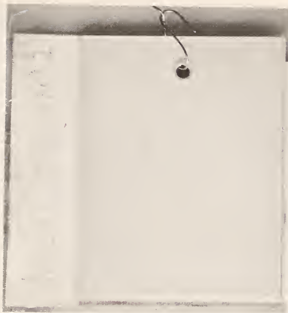
Figure 2. The back surface of a test specimen for the fungus resistance test. The right portion of the specimen shows the glass substrate to which the plastic wallcovering material was adhered. The left side of the test specimen, where the code number is written, is the area where the effect of fungi was evaluated on the backing material alone.
