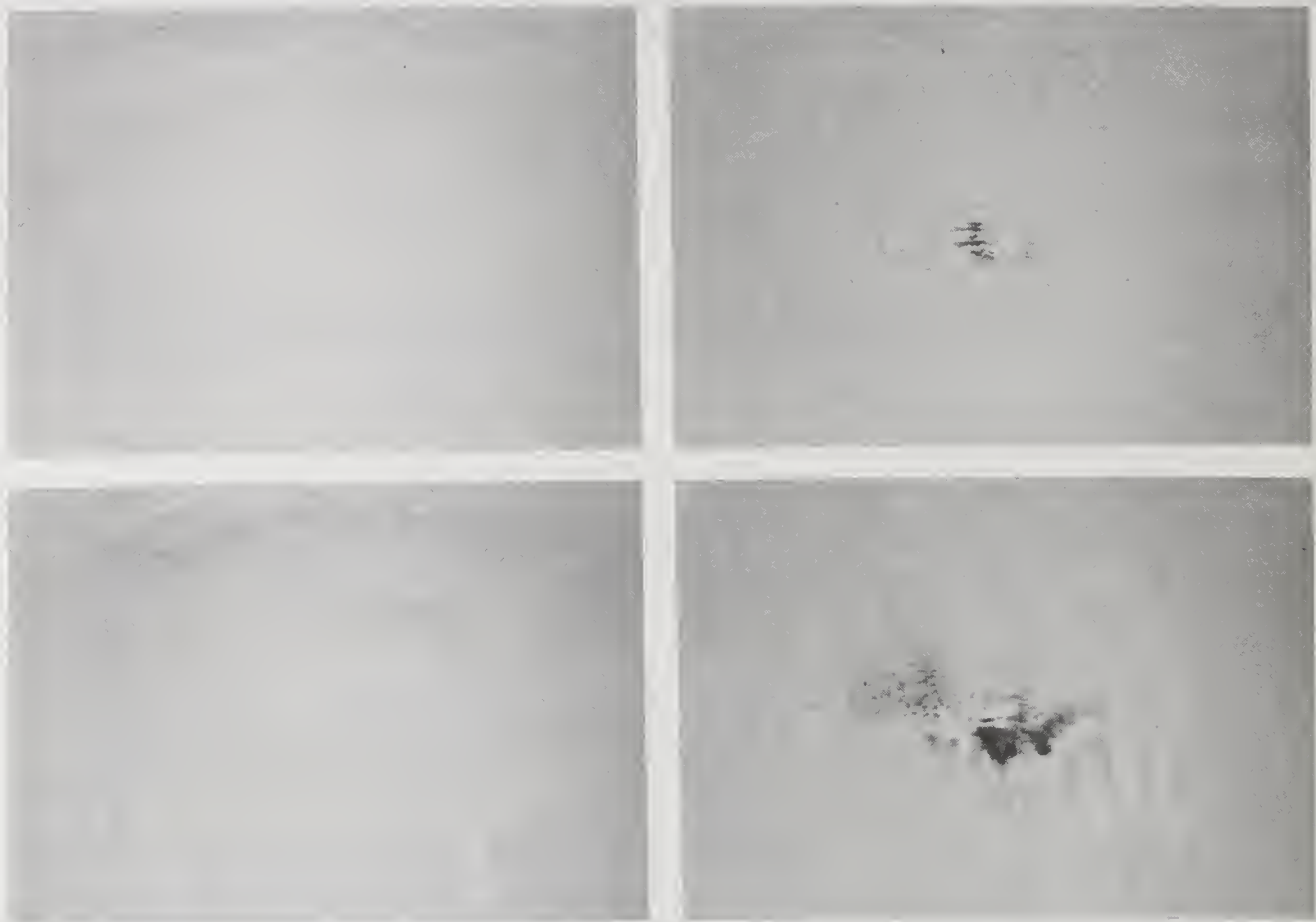
Fig 2 A sequence of schlieren images of a silicon surface
