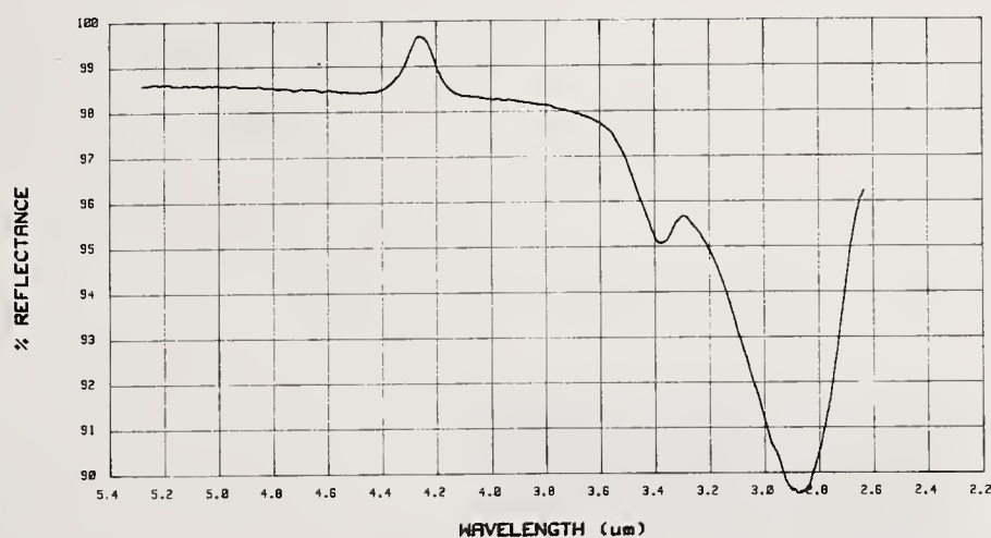
Figure 4. Plot of reflectance versus wavelength shown with wavelength decreasing from left to right for an undosed CaF 2 film on SPDM Cu. The sample has gone through a 12-hr bakeout. The reflectance minimum at 2.9 \mu m at around 89.5% is due to H 2 O. The additional local minimum at 3.4 \mu m is due either to loosely bound OH - or hydrocarbons. The bump around 4.3 \mu m is a calibration artifact.
