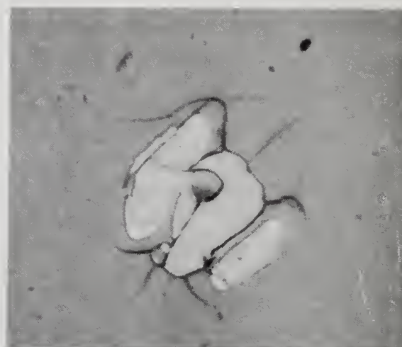
Figure 10. Photograph of HF laser-induced damage of undosed \text{CaF}_2 on quartz. Damage morphology is fracture and delamination; 360X magnification.
