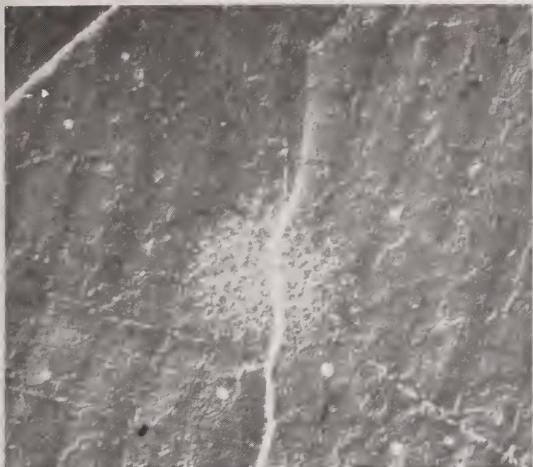
Figure 12. Photograph of HF laser-induced damage of H 2 O-dosed CaF 2 on SPD Cu. Damage morphology is ablation and "orange-peel-like" surface roughening; 360X magnification.
