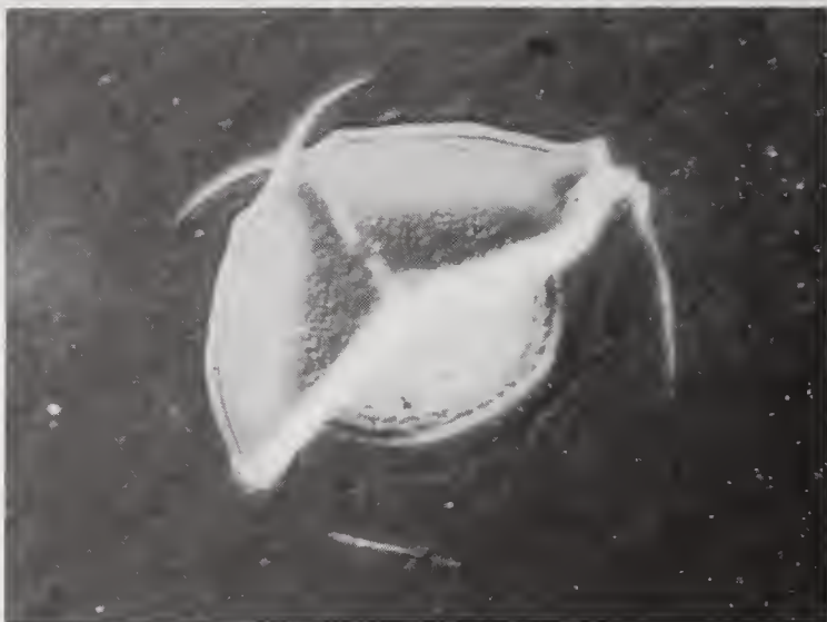
Figure 9. Photograph of HF laser-induced damage of undosed \text{CaF}_2 on SPD Cu. Damage morphology is fracture and delamination; 360X magnification.
