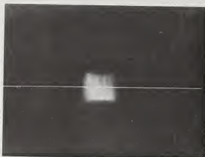
Figure 3. Intensity inverted video picture of CO 2 laser quenched fluorescence. The rectangular focal zone is approximately 5mm X 5mm.
