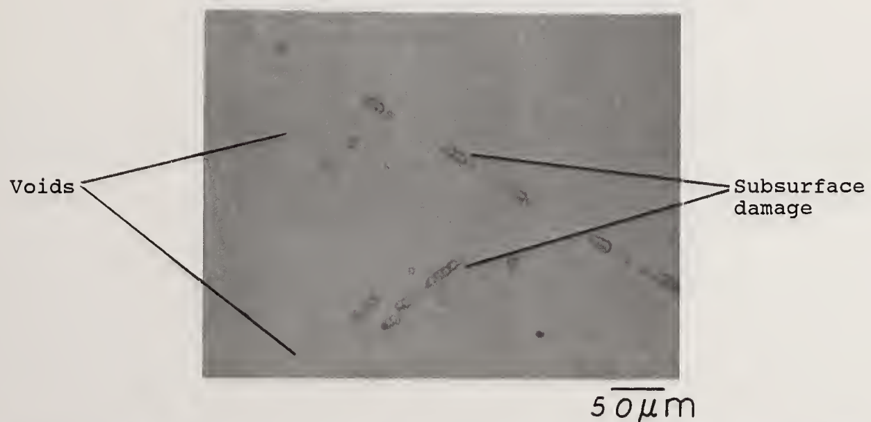
Figure 3. Nomarski micrographs showing representative subsurface defect on fused silica surface after exposure to selective delineation etch (a) super polish, (b) standard polish
