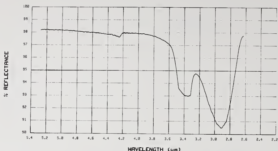
Figure 5. Plot of reflectance versus wavelength shown with wavelength decreasing from left to right for a D 2 O-dosed CaF 2 film on SPDM Cu. The sample has gone through a 12-hr bakeout. The reflectance minimum at 2.9 \mu\text{m} , up from the coating discussed in figure 4 at around 90.5%, is due to H 2 O. The additional local minimum at 3.4 \mu\text{m} has increased dramatically over the undosed film and has saturated the detector. No evidence of absorption related to the D 2 O dosing is evidenced.
